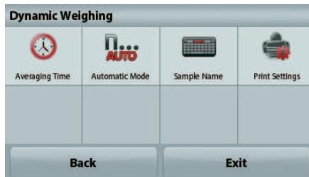
**Automatic Mode:** When set to On, the cycle begins when an object is placed on the pan, and the held value is automatically reset when the object is removed from the pan.
