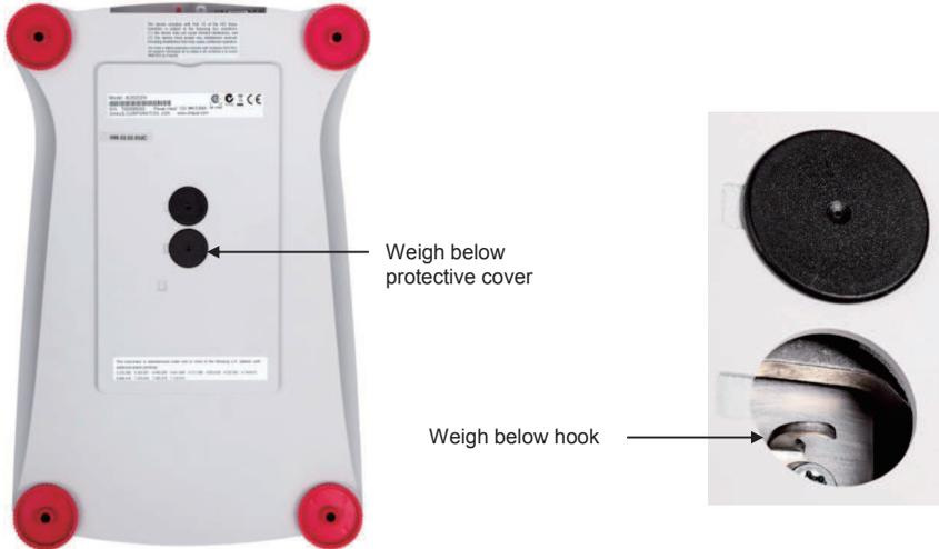
The balance can be supported using lab jacks or any other convenient method. Ensure the balance is level and secure. Power on the balance, then use a string or wire to attach items to be weighed.
