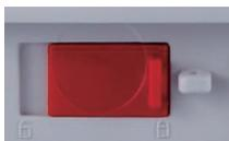
**Note:** The security switch located at the rear of the balance must be in the locked position to set Approved Mode to ON. The security switch must be in the unlocked position to set Approved Mode to OFF. See Section 6.
