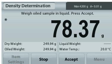
Once the necessary weights have been determined, the density of the sample is displayed in **g/cm<sup>3</sup>** (along with the weight in air, un-oiled and oiled, and weight in water) on the Application screen.
