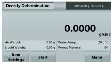
**Step 1 of 2 – Weigh the Sample in Air.** Press **Start**. Follow screen instructions, then press **Accept** to store the dry sample weight (“in air”).
