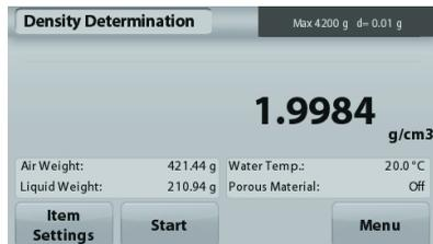
Once the necessary weights have been determined, the density of the sample is displayed in **g/cm<sup>3</sup>** (along with the weight in air, weight in water) on the Application screen.
