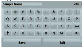
Key in the desired sample name and press Save to save the name and return to weighing home screen.
