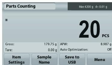
**Auto Optimization:** When set to **On**, improves counting accuracy by re-calculating the piece weight automatically as parts are added. Default is **Off**.
