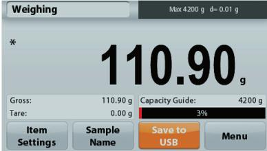
**Notes:** The first time a USB flash drive is connected to the balance there might be some delay time before the button **Save to USB** works. This is due to that the balance is creating the necessary folders on the USB flash drive where the data will be stored.
