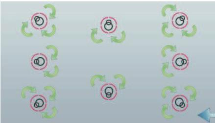
Rotate the feet according to the image above depending on the location of the level bubble until the bubble is centered.
