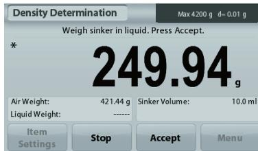
Once the necessary weights have been determined, the density of the Liquid sample is displayed in **g/cm<sup>3</sup>** (along with the weight in air, weight in water) on the Application screen.
