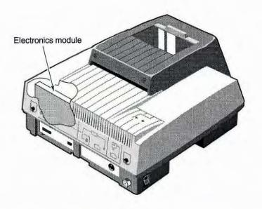
The electronics module inside the spectrometer could overheat. A
