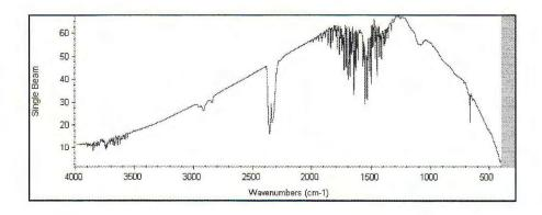
For most applications you don't need to collect a new background spectrum for each sample spectrum if you haven't changed the software parameters. To obtain good results, however, collect a new background regularly, perhaps once every four hours. (You can obtain the best results by collecting a new background for each sample, but this is seldom necessary.)
