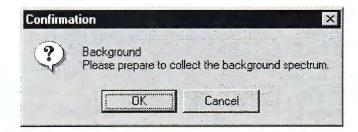
This means that you need to remove any sample from the sample holder so that the infrared beam path is clear.
