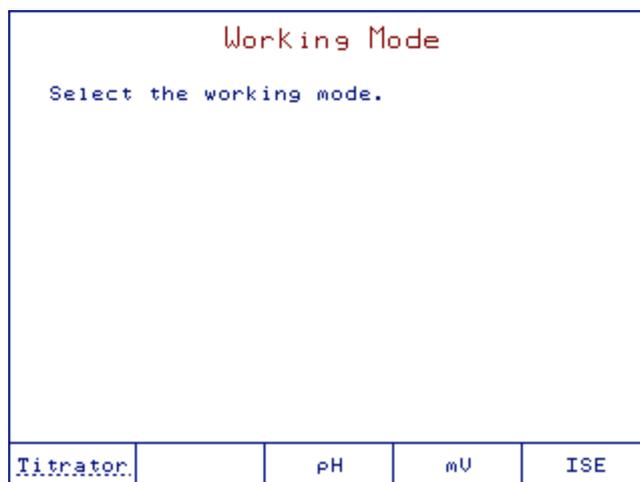
When one of these keys is pressed, the titrator will enter the selected mode:
