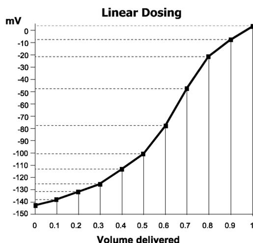
Linear dosing is recommended for titrations with a slower reaction rate, difficult nonaqueous titrations, and specific applications.
