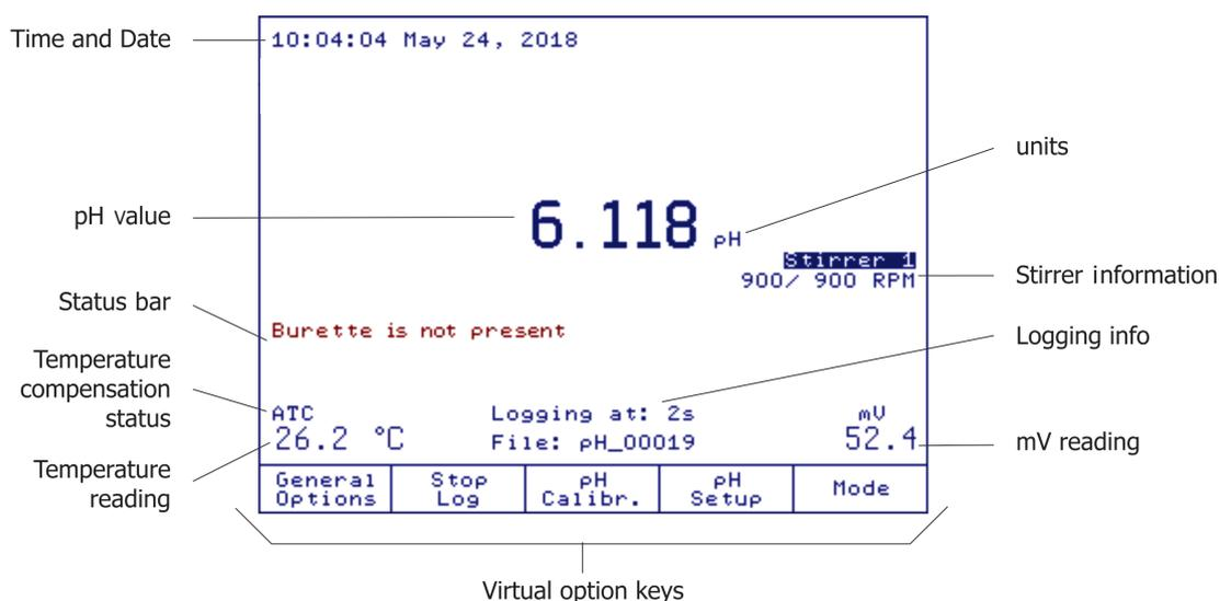
If one of these keys is pressed, the associated function is immediately performed. Some of the keys are active only in specific screens:
