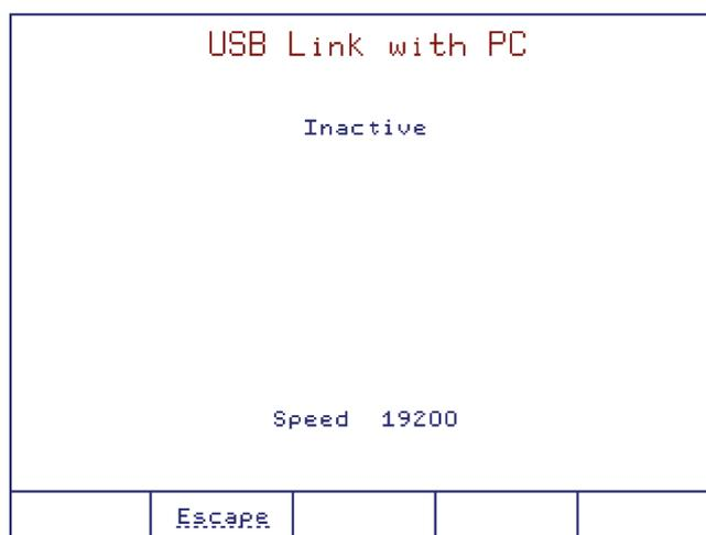
The **HI900** PC application allows the transfer of methods and reports between the titrator and PC. See **3.12. USB LINK WITH PC** section for more information.
