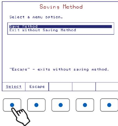
The **Saving Method** screen allows the user to save the modifications. To exit without saving, press **Escape** or highlight *Exit Without Saving Method* option and then press **Select**. To save the modifications, highlight *Save Method* option and then press **Select**.
