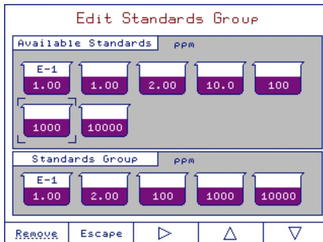
Use the arrow keys to select the standard to be included in / removed from the standard group.
