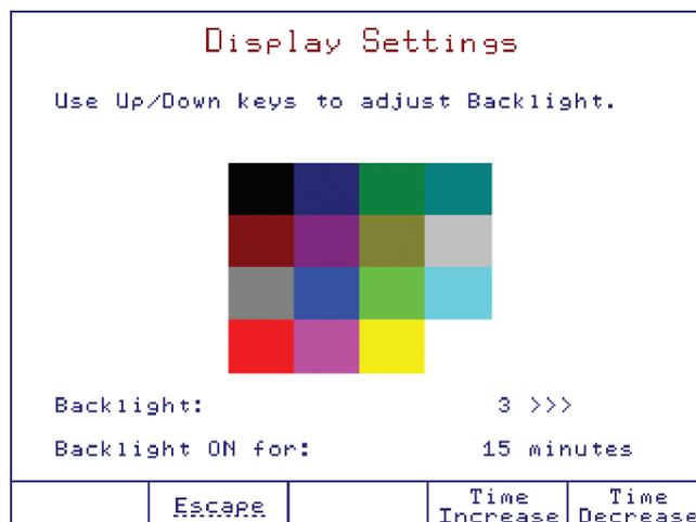
The displayed color palette allows for selection of appropriate backlight intensity.
