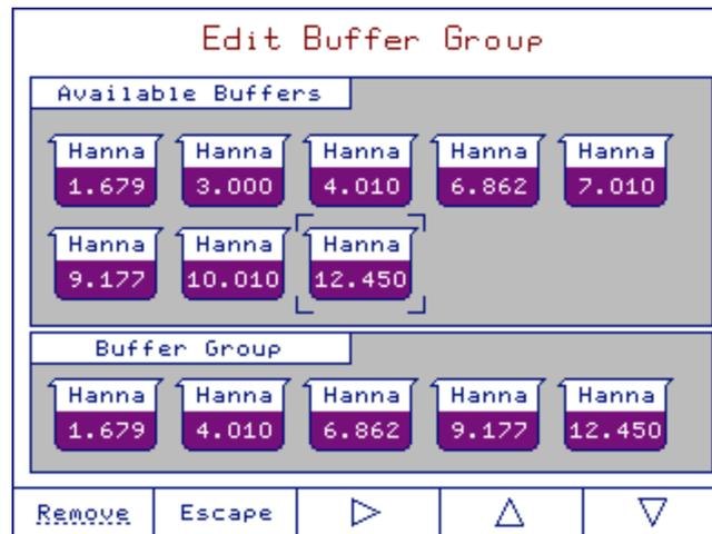
Use the arrow keys to select the pH buffer to be included / removed in / from the buffer group.
