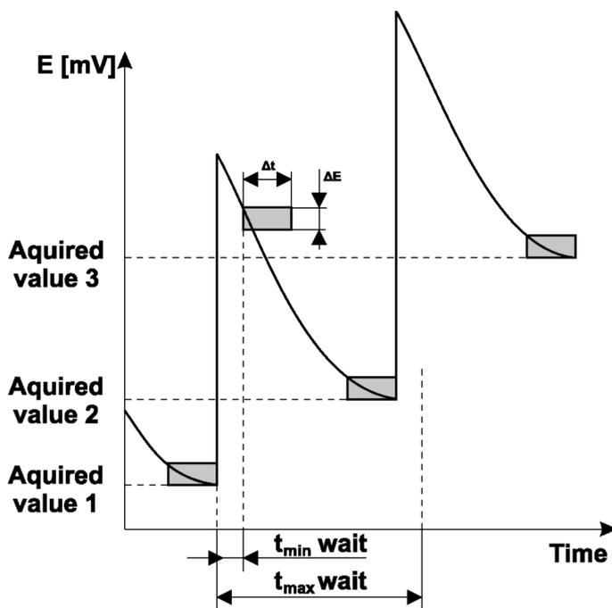
The signal stability window (condition) represents the time interval ( $\Delta t$ ) during which the potential measured in solution (mV) is confined inside the potential interval ( $\Delta E$ ).
