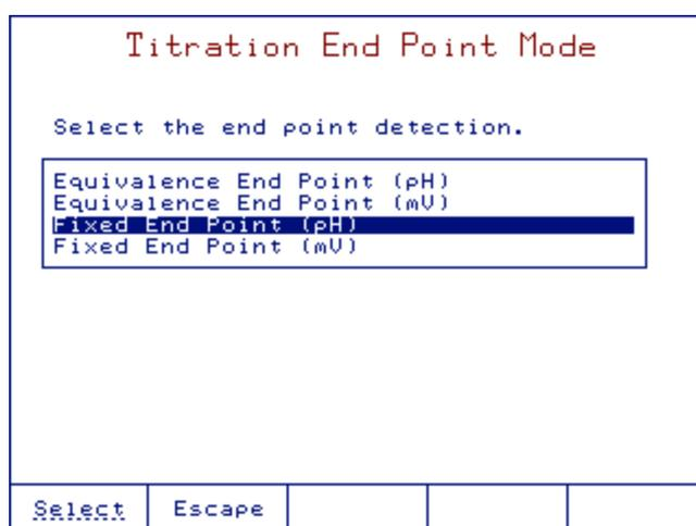
**4.5.6.1. Fixed Endpoint (pH or mV)****Fixed Endpoint (pH)**
