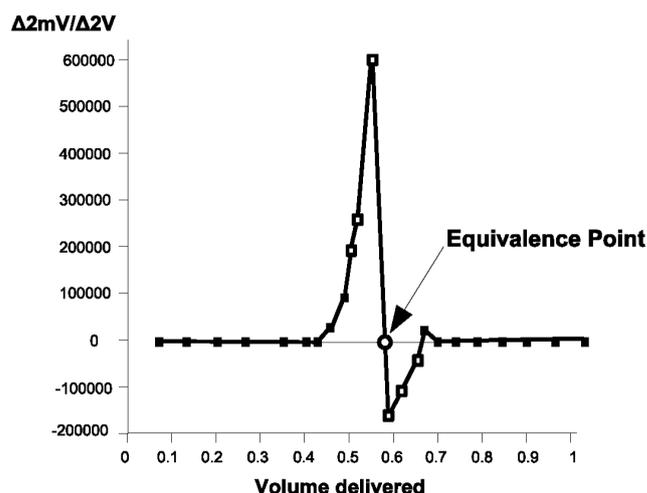
The detection algorithm looks for the point where the second derivative changes sign. The checked point, or 1<sup>st</sup> derivative, must be greater than the threshold value. See [4.5.7. RECOGNITION OPTIONS \(EQUIVALENCE ENDPOINT ONLY\)](#) section for more information.
