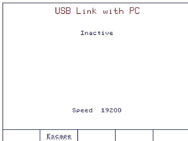
“Active / Inactive” message shows the status of the USB link with the PC.
