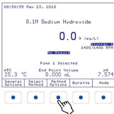
Press the option key below the virtual key. For example, to access the **Method Options** screen, press the option key below it.
