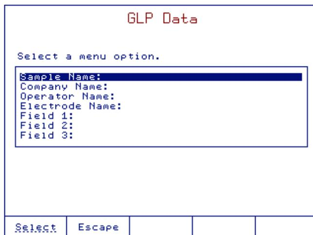
**Sample Name** Allows the sample name to be recorded in each report. The sample name will increase by one, with each new titration or logging report, if the last character is a number.
