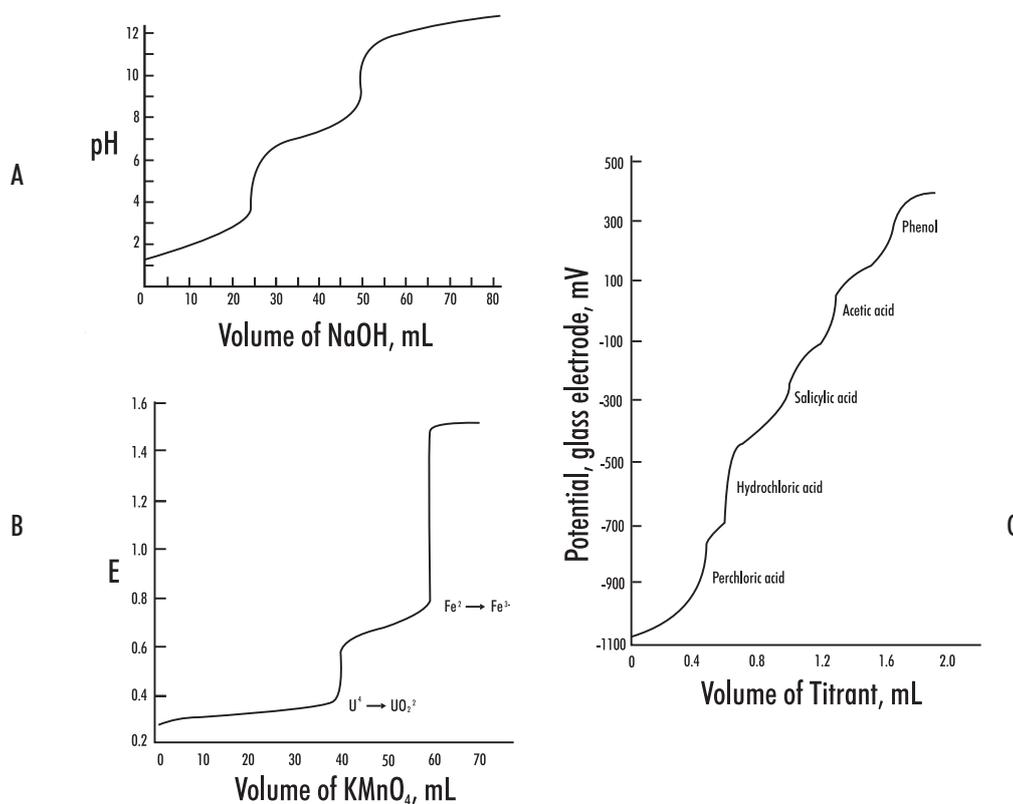
Figure 9: Multiple endpoint titrations
