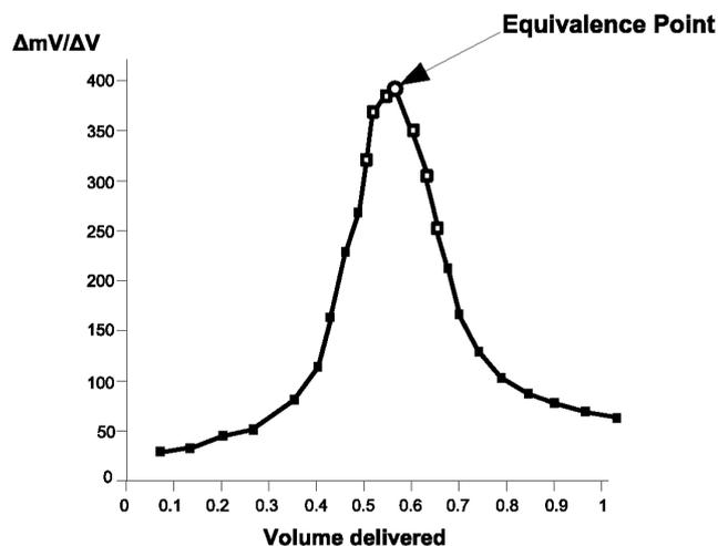
The detection algorithm looks for the maximum value of the 1<sup>st</sup> derivative. The 1<sup>st</sup> derivative must be greater than the threshold value at the maximum point. See [4.5.7. RECOGNITION OPTIONS \(EQUIVALENCE ENDPOINT ONLY\)](#) section for more information.
