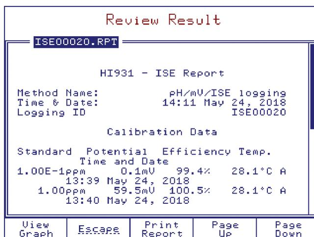
The report contains information based on the selections made in the **Setup Titration Report** and **Setup ISE / pH / mV Report** screen.
