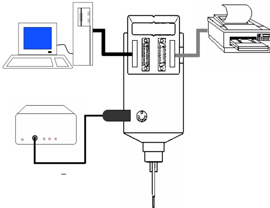
Figure 2-1 Interconnection Diagram
