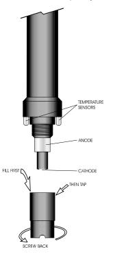
4. Whit the sensor facing down screw the cap clockwise to the end of the threads. Some electrolyte will overflow.
