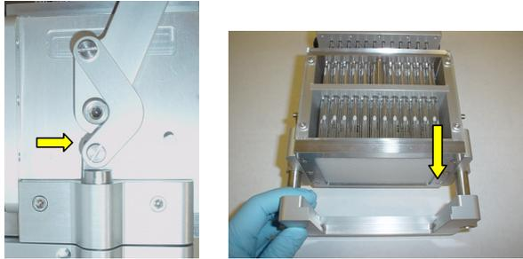
**Figure 5-8: Side view of Hydra syringe head flat head screws and bottom view of syringe head C Clamp to be removed.**
