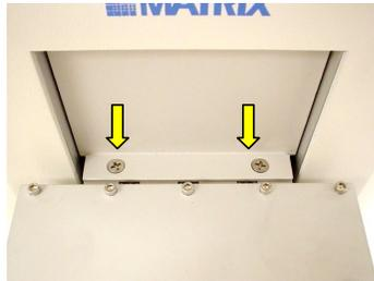
**Figure 5-3: Top view of the Hydra DT tower Philip head screws to be removed**
