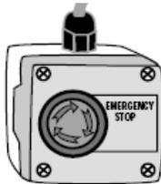
**Figure 2-8: Emergency Shutoff Switch**
