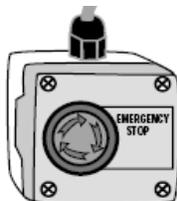
Figure 3-4: Emergency Shutoff Switch
