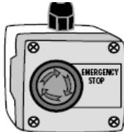
**Figure 7-1: Emergency Shutoff Switch**
