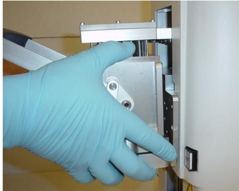
**Figure 5-6: Lifting the syringe head from the Hydra DT tower**
