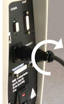
**Figure 2-7: Attaching E-stop plug**
