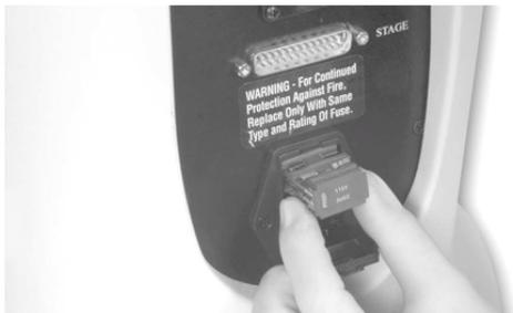
**Figure 5-18: Removing the Fuse Box**
