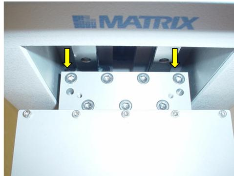
**Figure 5-5: Top view of the 7 socket head screws to be removed from syringe head**
