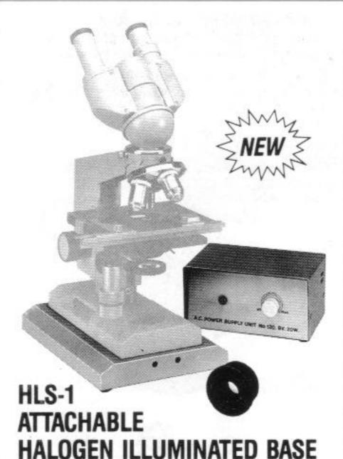
Designed to be easily fitted to the exisiting base-plate of all Biolam microscopes. It provides a high level of illumination, suitable for phase-contrast etc., by means of a 6volt, 20watt halogen bulb. Evenness of illumination is assured by a semi-ground condenser lens, and the level of illumination is controlled by a separate transformer/rheostat.
