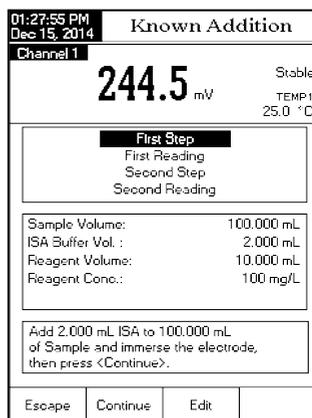
Start by adding 500  $\mu\text{L}$  at a time (for example). Watch the change in mV. When you have observed approximately a 15 mV change from the original sample, calculate the total volume added. Adjust sample and standard volumes proportionally to standard volumes that can be measured with accuracy. Use volumetric pipettes for standard, ISA and sample addition.
