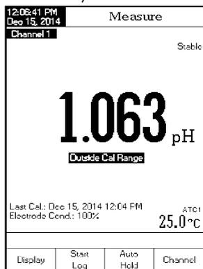
*Notes: For single channel pH measurements (HI5221), “MTC” or “ATC” indicators will be displayed on the LCD, while for dual channel pH measurements (HI5222) “MTC1”/“MTC2” or “ATC1”/“ATC2” indicators will be displayed (Channel dependent).*
