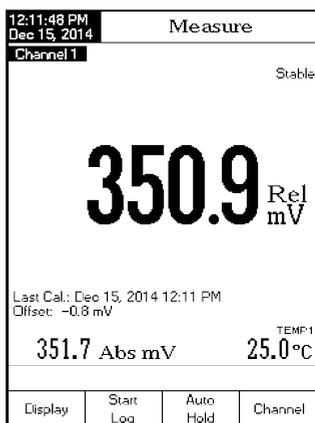
For greater accuracy, it is recommended to calibrate the ISE sensors frequently. The instrument should be recalibrated when "ISE x Calibration Expired" (the "x" represents channel "1" or channel "2") message appears on the LCD, in the Reminder messages area.
