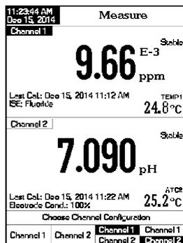
For each measurement mode (pH, mV, Rel mV or ISE) the following display configurations are available: Basic, Good Laboratory Practice (GLP) (pH, ISE only), Graph and Log History.
