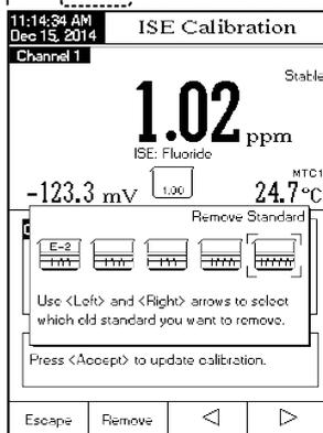
Press  to delete the selected calibrated point and then press  to update calibration with the new standard solution.
