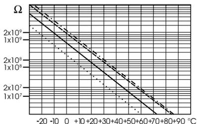
Since the resistance of the pH electrode is in the range of 50 – 200 MΩ, the current across the membrane is in the pico Ampere range. Large currents can disturb the calibration of the electrode for many hours.
