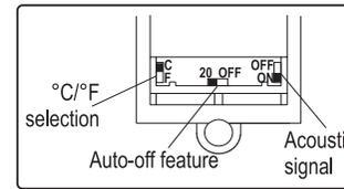
To access these features, remove the battery cover on the back of the meter and extract the battery. Select the desired settings, insert the battery and close the cover.
