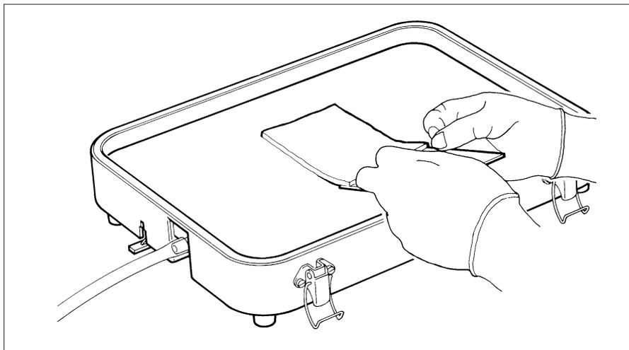
5. Starting with one of the gel edges, gradually slide the gel from the support plate onto the membrane to fill the window. As necessary, position the part of the gel carrying the sample wells accurately on the line drawn on the mask (see Section 4.1).
