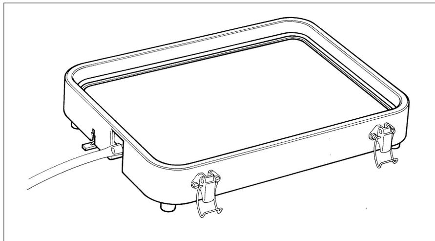
2. Prewet the porous support screen in distilled water and place it on the inner rim of the base unit with the shiny side up.
