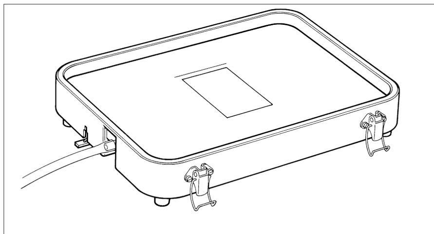
3. Place the plastic mask with the window on the support screen.
