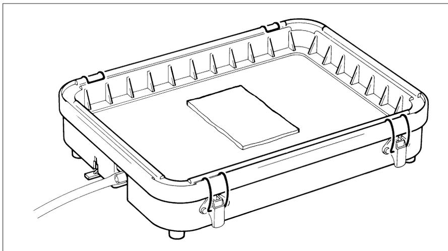
6. Fit the top frame and secure it by tightening the four clamps. Switch on the vacuum pump to immobilize the gel.
