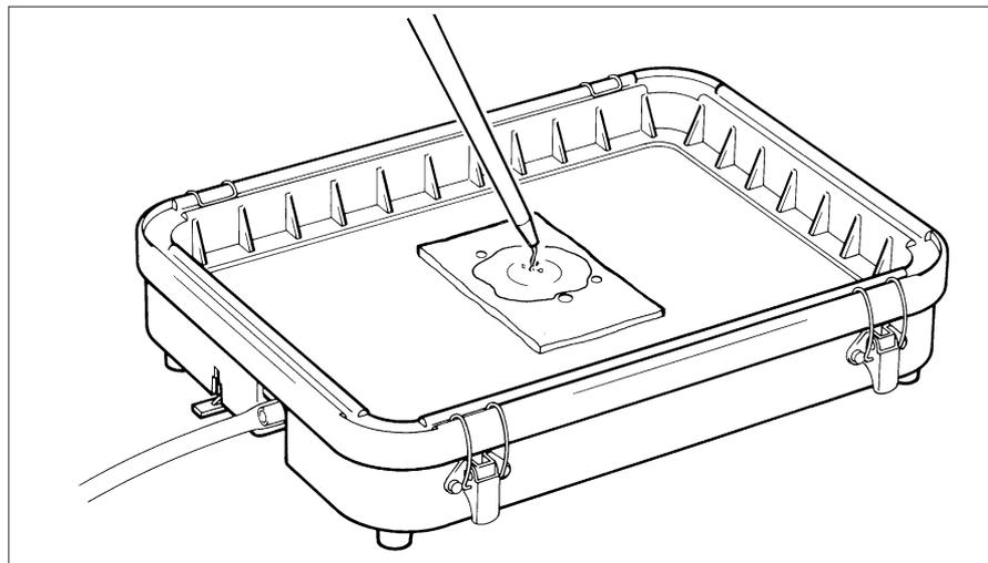
7. Without waiting for the vacuum to reach the working level, pour Solution 1, Depurination Solution, onto the centre of the gel. Use enough solution to cover the gel. Leave for 7 minutes. Ensure that the gel remains covered with solution during the treatment.
