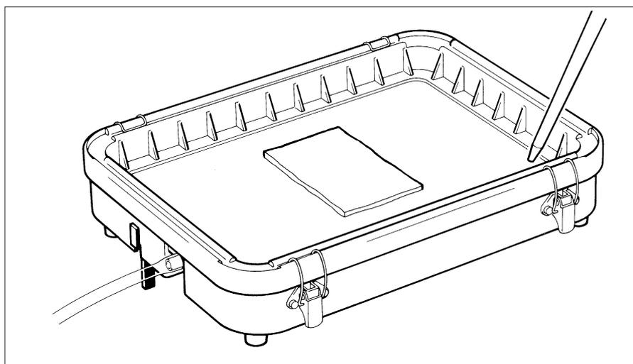
9. After 7 minutes tilt the blotting unit using the collapsible stand. Remove residual liquid on the gel by gently wiping over the surface with a gloved finger. Remove liquid from the base unit either by pipette or by using vacuum suction. The vacuum pump can be utilized for this purpose by coupling a t-connector to the tubing between the blotting unit and the liquid trap. Make sure the liquid suction outlet can be closed when not in use.
