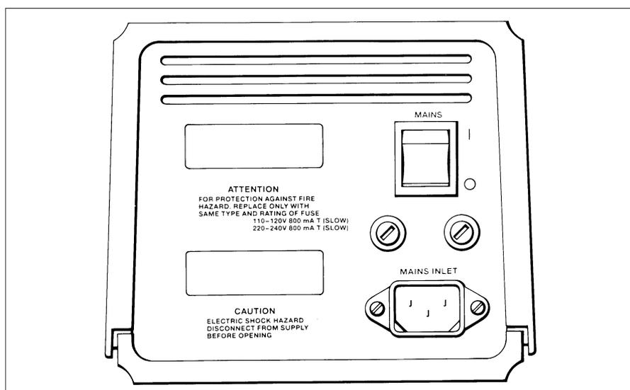
1. Check that the main power switch on the back panel of the pump is OFF, in the 0 position.
