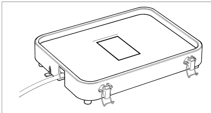
4. Position the pretreated transfer membrane under the mask so that it covers the window in the plastic mask completely. Make sure no air bubbles are trapped in between the membrane and the porous support screen.
