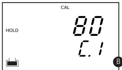
2. **Press the ENTER key** to begin calibration. The “CAL” indicator will appear on the display. The upper display will show 80. The lower display will show C1 (= calibrated value 80%).
