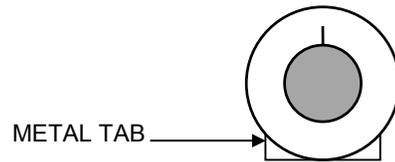
Rotate both knobs—speed control and timer—to their extreme counterclockwise positions before connecting unit to power source. After inserting the plug, press all switches to the unlit **OFF** positions; then turn on power switch. It will light to indicate that power is **ON**.
