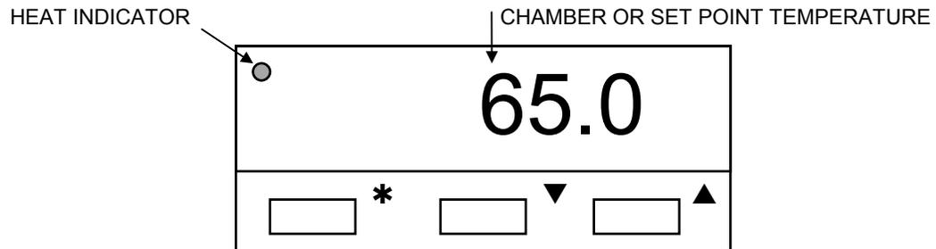
1. **CONTROLLER SELF-TEST:** When the incubator is powered up the controller will display **8888** along with the three decimal points and the heat **ON** indicator lamp. The display will then blank out for 2 seconds before showing the chamber temperature.
