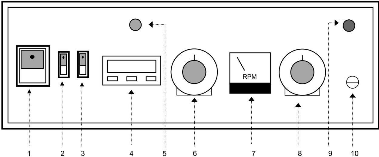
1. **POWER SWITCH:** A 2-position switch that turns on power to the unit.
