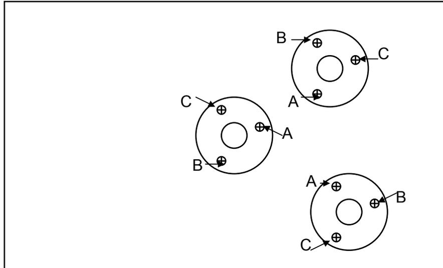
3 PHILLIPS SCREWS AT EACH OF 3 BEARING MOUNTS = 9 SCREWS
