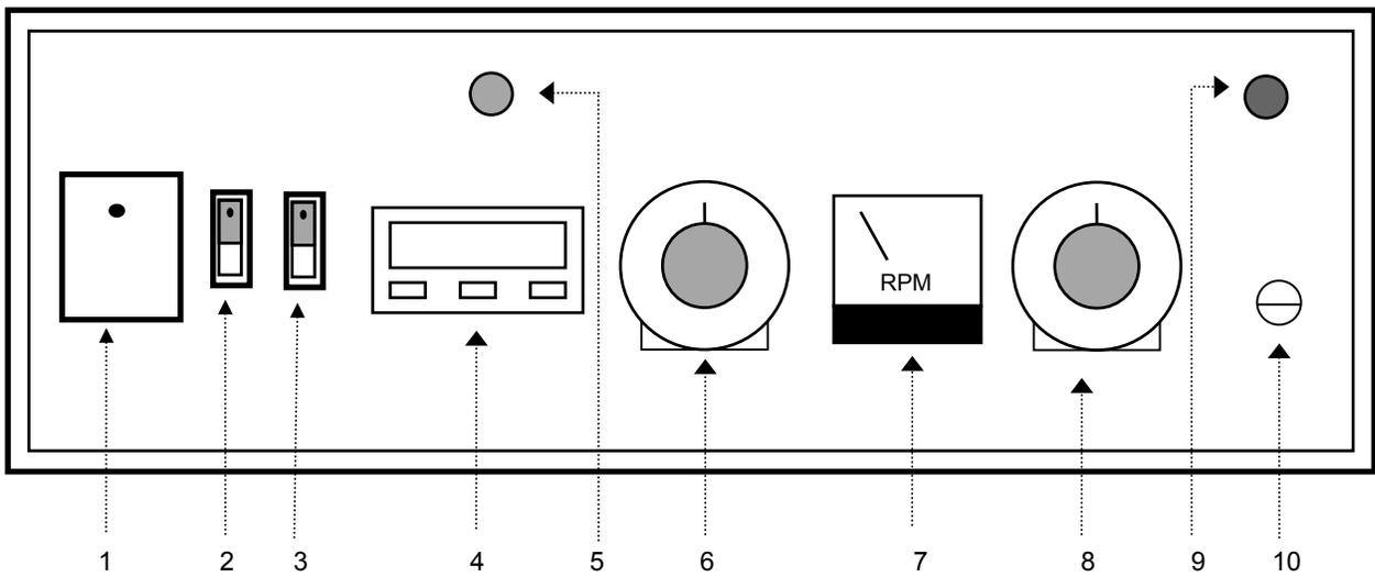
8. **TIMER:** The control can be used to set a timed shaking cycle from 1 to 60 minutes or to run continuously.
