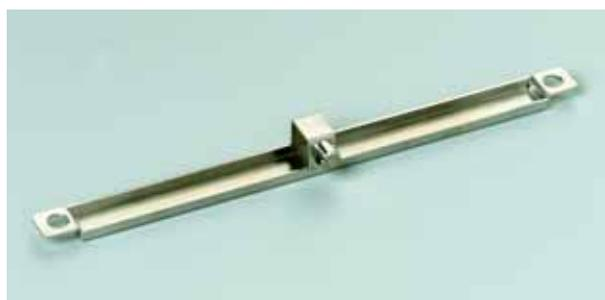
The drop catcher is carried by the upper side of the magnet unit and is placed directly below the nozzle head each time it moves anywhere except from one well to the next. If a drop should leave the pipet, it is caught by the drop catcher.
