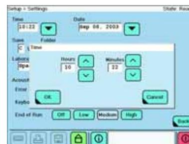
**8b** Touch the Up and Down buttons (to the right of each number) to change the values for year, month and day (see figure). The Up button increases values; the Down button decreases values. Touch the OK button to confirm the changes and return to the SETTINGS Screen. Touch the Cancel button to return to the SETTINGS Screen without changing any settings.
