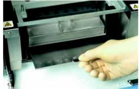
To remove and place the Liquid Drop Catcher on the magnet unit, first remove the Cartridge Rack:
