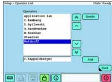
To enter a new operator type a new name into the entry field below the Operator List and select the Add button.
