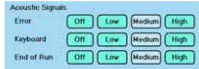
Note: You can choose to sound an alarm each time an error message is displayed (Error), each time a button has been touched on the virtual keyboard (Keyboard), and each time the purification run has ended (End of the run). If you don't want one of these alarms, just select **Off** for that particular alarm. For each alarm you want, choose whether the alarm sound should be given at low, medium or high volume.
