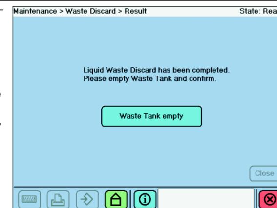
Always empty the Waste Tank after each purification run, when asked by the instrument's software to do so, or the instrument might be severely damaged! Treat the liquid waste as biohazardous material. Empty and clean waste tank as described in chapter C 3.1 Cleaning. If the Waste Tank should overflow, it is essential to clean the instrument according to the local regulations.
