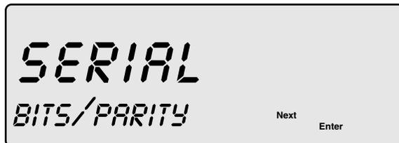
2. Press "Next" to scroll through selections (8-none, 7-even, 7-odd and 7-none) and press "Enter".
