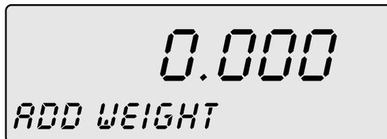
2. Place mass standard on the weighing pan (see Permissible Weights at the end of this section). The balance recognizes the mass and automatically calibrates.
