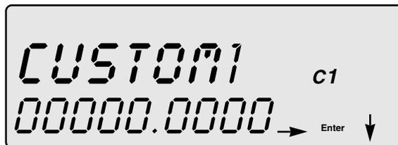
6. Enter the desired factor using the arrow keys.
