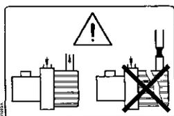
Warning - do not block the pump outlet.
