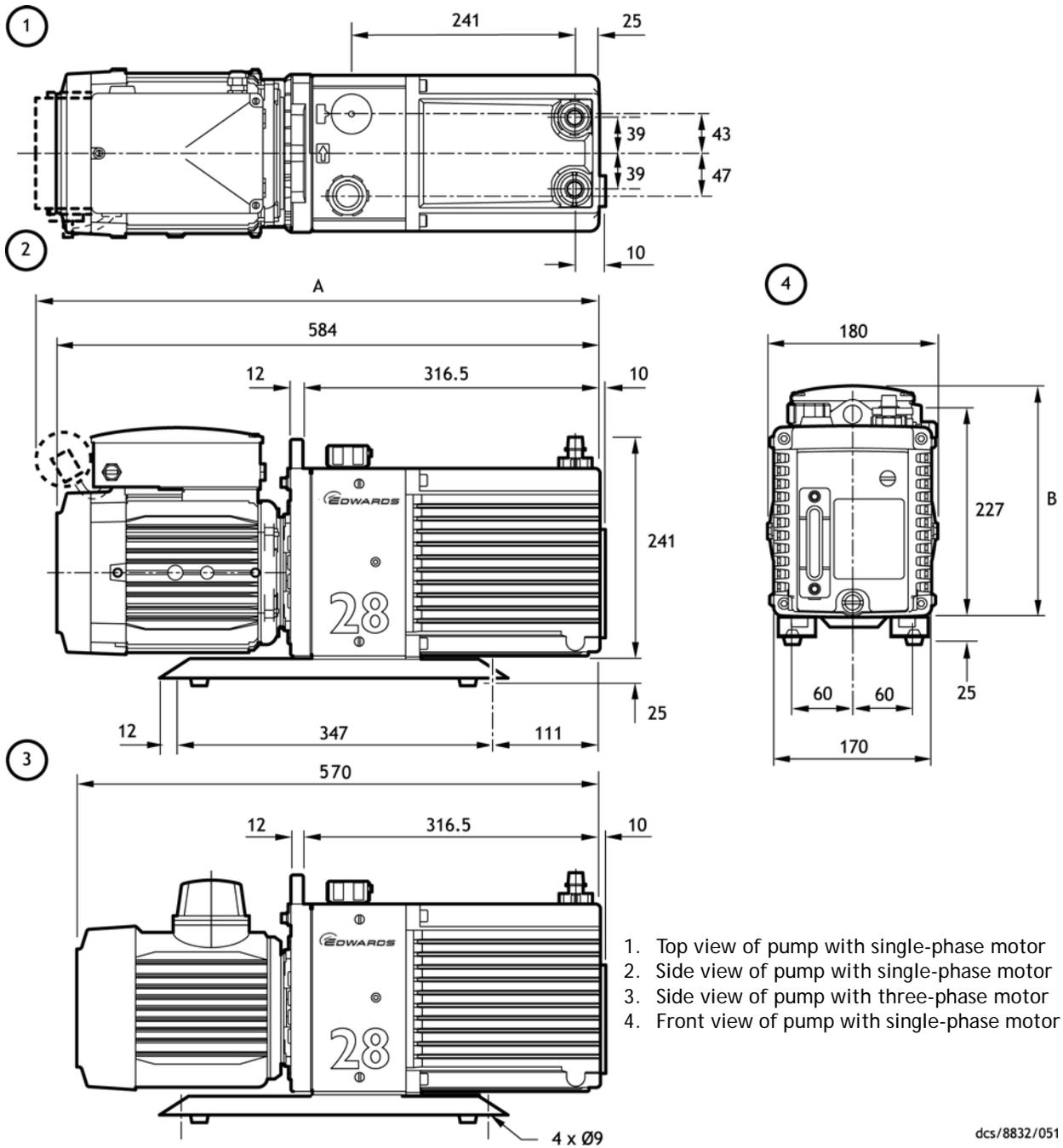
1. Top view of pump with single-phase motor
