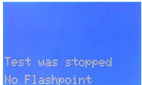
OVERFLO 10°C above the pre-set temperature of the expected flashpoint the program automatically is aborted for safety reasons.
