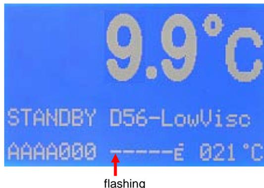
Now it is possible to put the precooled sample into the crucible. Having inserted the crucible into the heating block the test can be started by RUN. To prevent the empty heating block from icing-up we recommend to cover it with appropriate isolating material during cooling.
