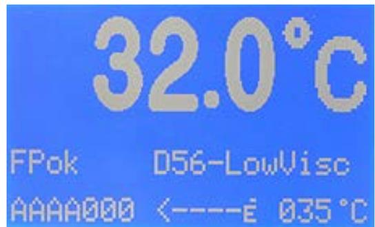
The device automatically cools down to auto start temperature.
