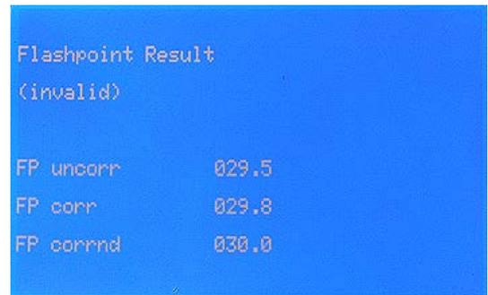
FPnoP02 The flashpoint was detected by a non-standard test. The pre-set cryostat temperature was too high so the auto start temperature could not be achieved or using devices with air conditioning the auto start temperature cannot be achieved because the ambient temperature is too high.
