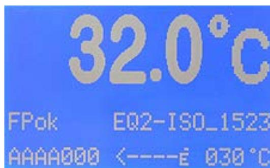
As a result the barometric pressure corrected, to 0.5°C rounded flash point is displayed.
