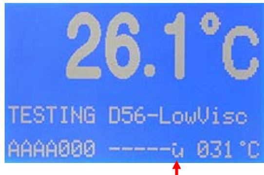
Flashpoint detected, ventilator turned on, block is cooling down.
