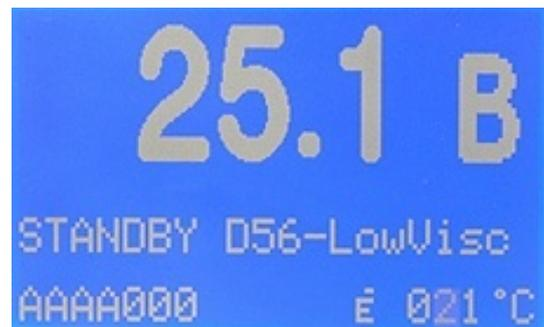
The flashing cursor is on the decimal digit of the flashpoint preselection.
