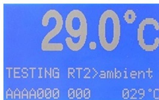
The result is similar to the test conduct in RT1<ambient either "noFP" (no flash point) or FPInval (flash point).
