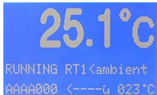
After auto start temperature was attained the device heats up to 3°C below the expected flash point:
