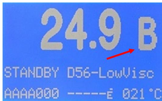
Sample temperature cannot be indicated. Heater block temperature is displayed and indicated by a "B" behind the value.
