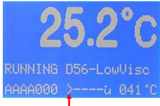
Device is testing for flash point. Cup symbol is flashing.
