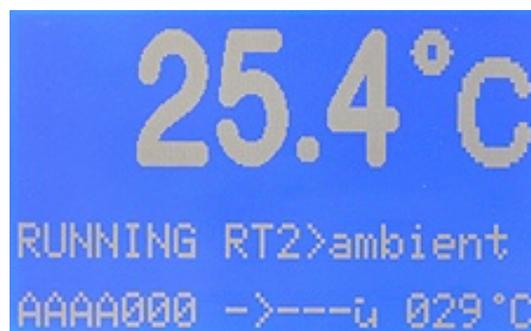
After reaching the test temperature there will be an acoustic sound for filling the sample with the syringe into the cup.
