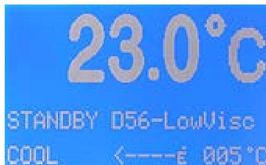
When the temperature goes below the threshold, the signal switches off. On the display "COOL" remains until the <STOP> key is pressed.
