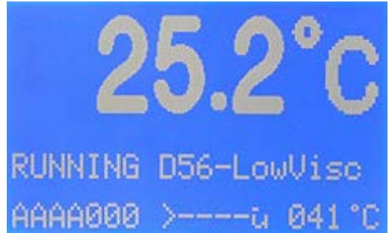
After achieving autostart temperature or directly after test start the ignitor glows for 30s for detecting ignitor reference voltage. Depending on the selected program the device gets into the test phase approx. 5°C before the preselected flashpoint. About 0.5 °C before first immersion there will be a short acoustic signal.
