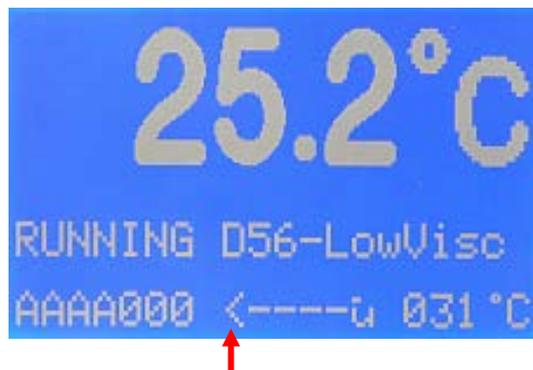
This test conduct is possible with pure materials. Working with mixed compounds the sample should always be cooled down to the temperature recommended by standards.
