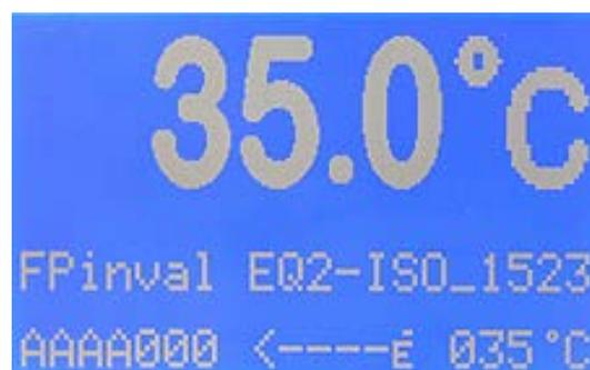
If no flash point is detected the sample is heated with 0,3°C/min and flash point tests are performed each 0,5°C.
