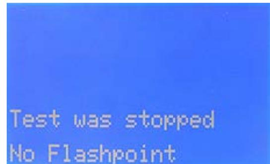
If no flash point is found in the 1. test according to ISO 1516 a further 10min temperating of the sample takes place:
