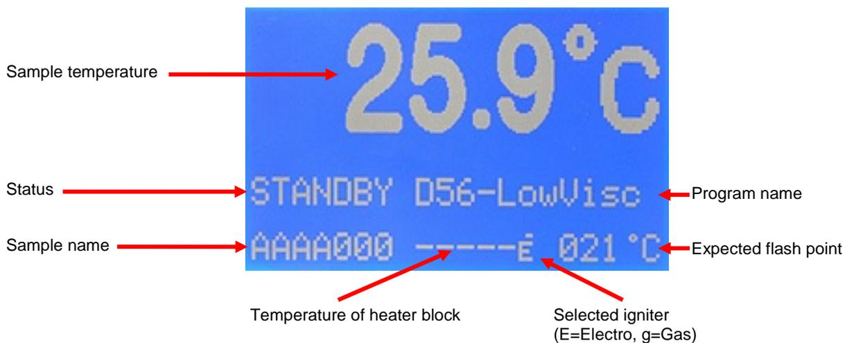
If TAG 4 is switched on without the test insert with indicator and sensor being assembled you will be given the following display:
