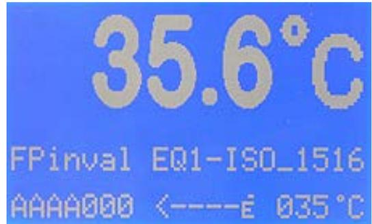
On the display the barometric pressure corrected, not rounded flash point appears. FPInval (invalid) shows that the test should be repeated at a lower temperature.
