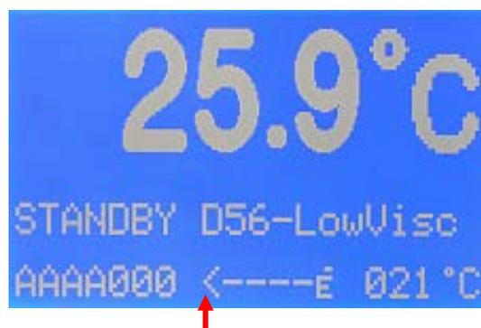
The block will be cooled down to auto start temperature (in the standards 11°C below expected flashpoint). This temperature will be kept for 5 min.
