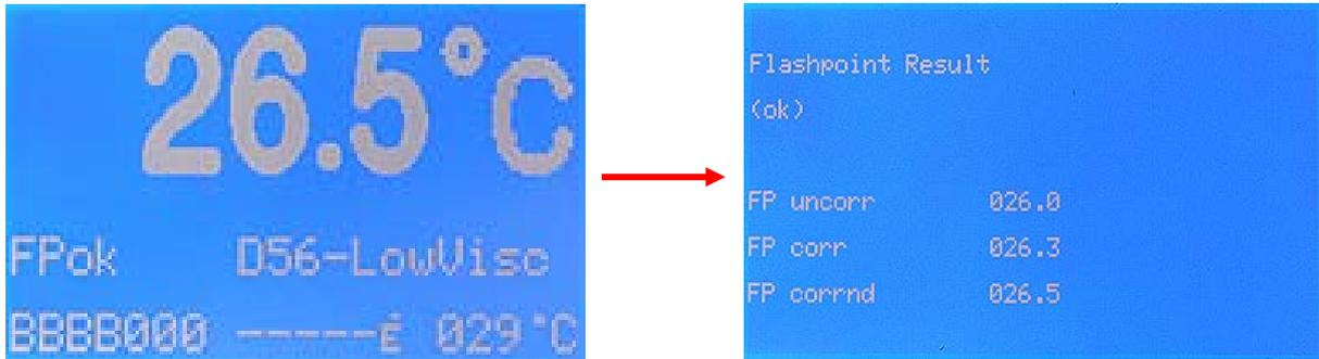
On the left (main) display always the barometric corrected rounded flash point is displayed.
