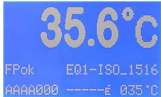
To switch between test conduct according to ASTM D 3934 and ISO 1516 program parameter 30 is set to 0001 (ASTM D 3934, preset as standard setting) or 0002 (ISO 1516).
