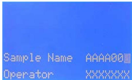
For sample- and user-ID you are given 7 digits which can be used for alphabetical (A to Z) or numerical (0 to 9) signs.
