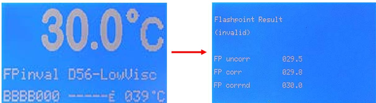
The test has to be repeated with a new sample and a flashpoint preselection at least 10°C lower than before.
