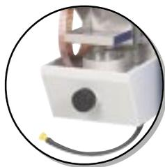
Safety features include a heating chamber with low voltage, high efficiency heating element and an automatic fire extinguishing system based on enhanced ultraviolet principles. A liquid trap prevents fire risk on the bench, while a drain tube facilitates easy cleaning.
