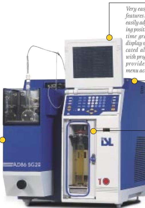
Very easy to use, the instrument features a graphic display that easily adjusts to an ideal working position and provides real time graphic and numeric display of test progress. A dedicated alphanumeric keypad with programmed function keys provides easy, instantaneous menu access.
