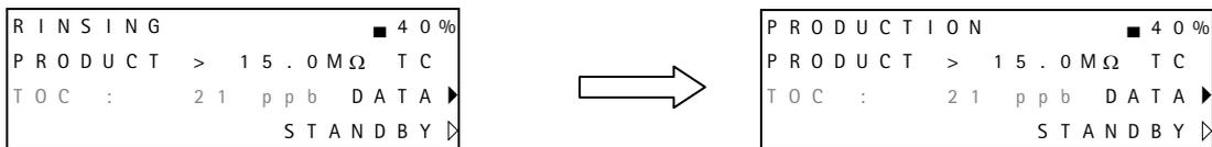
When a **Polisher is added to an Elix System**, the existing System Resistivity Sensor is used. When a Polisher is added, the existing Resistivity Sensor is configured to measure the Resistivity of the Post QGard Polisher Water instead of the post Elix Module Water. In the example displays above, the Polisher increased the resistivity from 13.1 MΩ.cm to > 15.0 MΩ.cm (at 25 °C).
