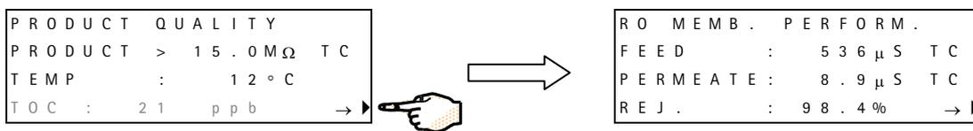
5. When the RO Cartridge performance is shown, press the Bottom Keypad Button to see the PRESSURE DATA.
