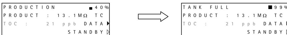
When the word **PRODUCT** appears on the 2nd line, the Resistivity and TOC values are measured inside the Elix System.
