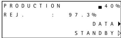
Pressing the Keypad Button next to STANDBY for a few seconds changes the LCD.
