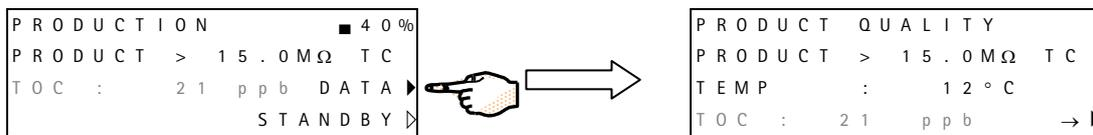
The post QGard TL Polisher resistivity is > 15.0 MΩ.cm at 25 °C. The same water has a temp. of 12 °C.
