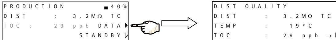
The Loop Water has a resistivity of 3.2 MΩ.cm and a TOC value of 29 ppb. The Loop Water has a temp. of 19 °C.
