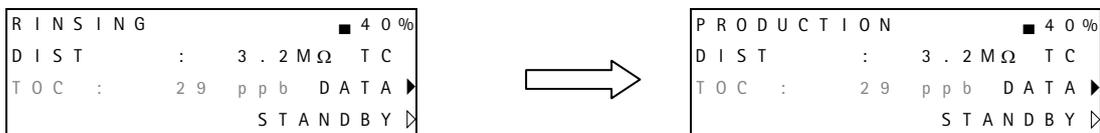
When **DIST is shown on the 2nd line**, then the Resistivity and TOC values are measured from the Loop Water. In the example shown immediately above, the water in the Loop has a Resistivity of 3.2 MΩ.cm (at 25 °C) and a TOC value of 29 ppb. In this same example, pressing DATA will then show the Resistivity and Temperature of the Elix System Product Water (the water filling the storage reservoir that becomes the Loop Water).
