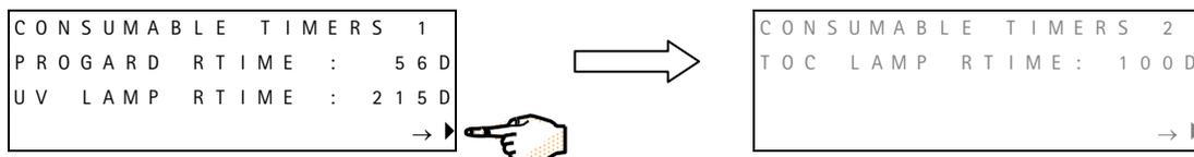
In this example, the A10 UV Lamp will need to be replaced in 100 Days
