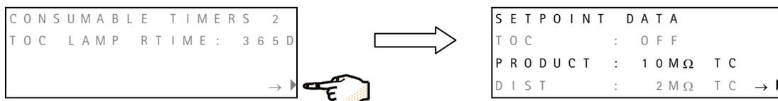
There are 3 Setpoints in the example shown immediately above. The TOC Setpoint is turned off. The Elix System Product Water Resistivity will turn on a message if its resistivity is < 10.0 MΩ.cm. The Loop Resistivity Setpoint is 2 MΩ.cm. A message will be displayed if the Loop Water Resistivity is < 2.0 MΩ.cm.
