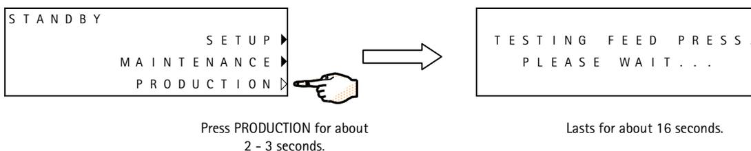
3. The Elix System will perform a Pressure Test for about 16 seconds. This tests the pressure reaching the Elix System.
