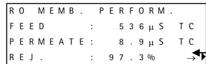
Pressing this Keypad Button (→) will scroll the LCD to the next LCD Screen containing DATA information. In this example, DATA is the Software Branch linked together with LCD Screens and the Keypad Arrow shown above.
