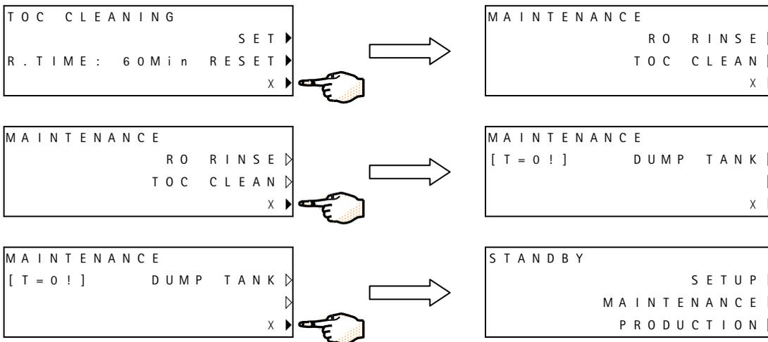
If the A10 TOC Monitor is measuring the TOC of the Elix System Product Water before entering the Storage Reservoir, then the TOC CLEANING Mode will start when the system enters PRODUCTION Mode.
