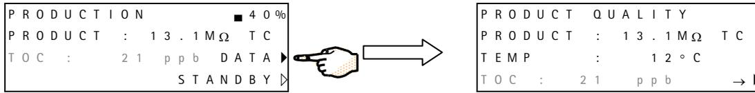
The Elix System Product Water Resistivity is 13.2 MΩ.cm. at 25 °C. The TOC is 21 ppb.
