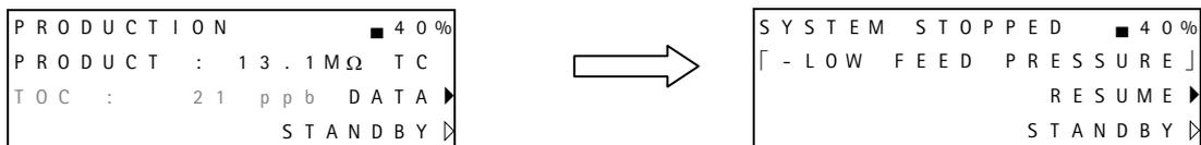
2. When the cause of the Alarm Stop Message has been corrected, press RESUME to go back to PRODUCTION Mode.
