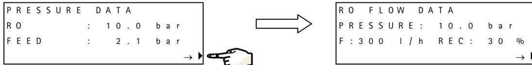
The Feedwater flow rate is 200 LPH. In this example, an Elix 70 was used and the calculated System Recovery is 30%.
