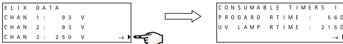
In this example the Progard TL needs to be replaced in 56 days and the Elix System UV Lamp needs to be replaced in 215 days.
