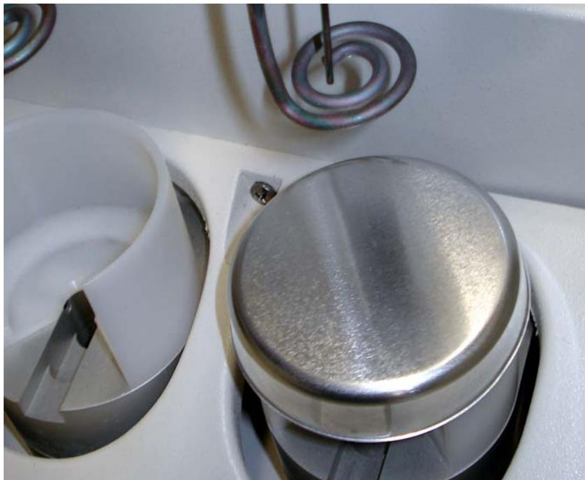
Cover the cradle when cleaning heaters, to keep the sensors and the tube flag in optimal condition.
