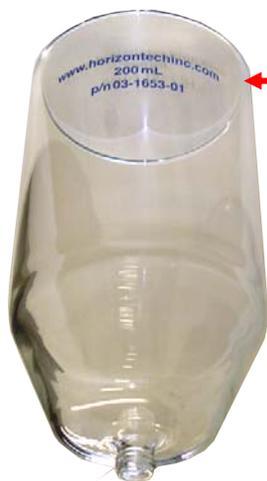
**200 mL EV Tube with GC vial thread**
