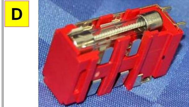
Turn the fuse holder over to access the fuse.
