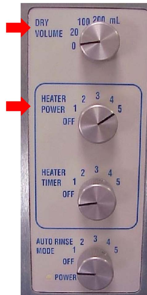
Fig. 3-4a Master Control Panel
