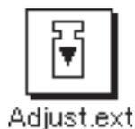
Pressing this function key triggers an adjustment of the balance using an external adjustment weight. You can do this at any time; you can also specify in the system settings that the balance requests adjustment as soon as a specified change in ambient temperature has taken place ("CallInfo" setting, Section 5.3.1). **Note:** Depending on regulations that vary from country to country, adjustment with an external weight may not be available on certified balances.
