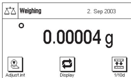
**Switch on the balance:** Switch the balance on by briefly pressing the "On/Off" key. Immediately after being switched on, the balance runs the most recently used application.
