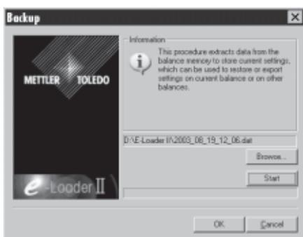
The dialog box opposite prompts you to select the path for saving the backup file through the "Browse" button. e-Loader II suggests a combination of the current date and the current time as a name for the backup file, and the file extension ".dat". (For example: "2003\_08\_19\_12\_06.dat" for backup file that was created on the 12th August 2003 at 12.06.) You are free to alter the file name, if you wish, but not the ".dat" extension.
