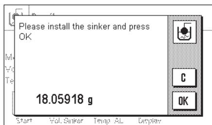
Press the **"Start"** function key to start the density determination. You are prompted to attach the sinker (weighing in air).
