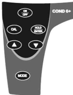
**ON/OFF** Powers meter on and off. Meter starts up in the measurement mode that you last switched off from.
