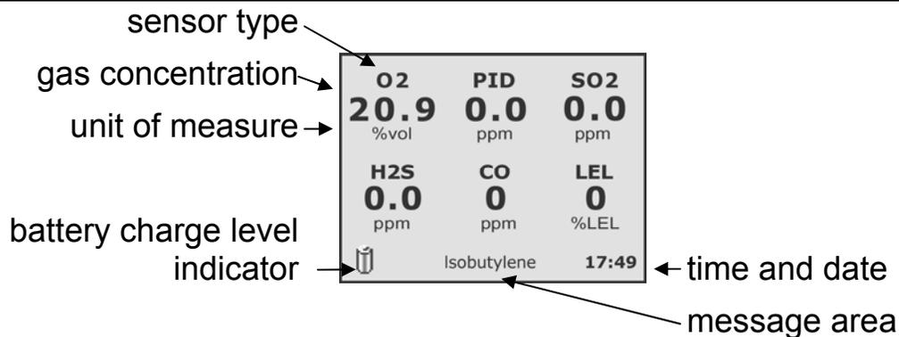
NOTE: The sample gas monitoring display screen is shown here in numeric format. Depending on the unit's configuration, some items may not display or may display differently.
