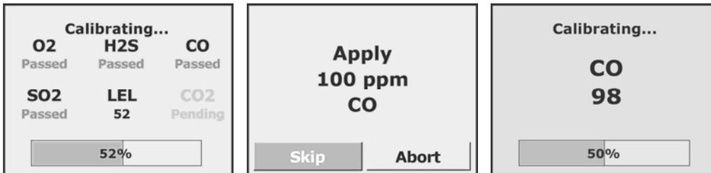
When the calibration is finished, the following screen shows the passed, marginal, skipped, and failed sensors, when six sensors are installed.
