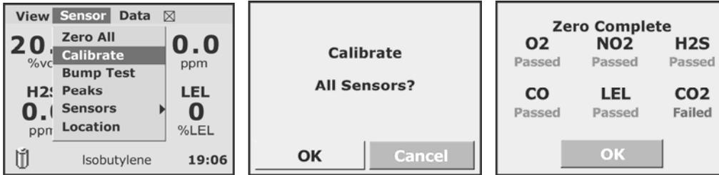
The screen to alert the user to connect gas to the instrument is then shown. Once the sensor starts to read gas, the calibration begins. The user has 5 minutes to apply gas before the calibration times out. Gas should be applied at a flow rate of 0.5 lpm. If the user chooses to “Skip” a sensor, the instrument will move to the next sensor. The “Abort” option aborts the calibration and shows the “Calibration Complete” screen.
