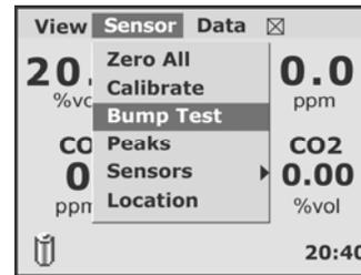
The unit asks the instrument operator to confirm the bump test request. If “Cancel” is selected, the user is returned to the gas-monitoring display screen. If the user selects “OK”, all the installed sensors are bump tested, starting with the first sensor.
