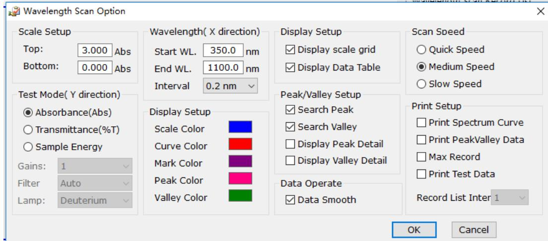
3. Select display mode (elected to the energy scan mode, the proposal is set to a fixed gain), scanning the wavelength range, coordinates the upper limit, lower limit coordinates and scanning interval.
