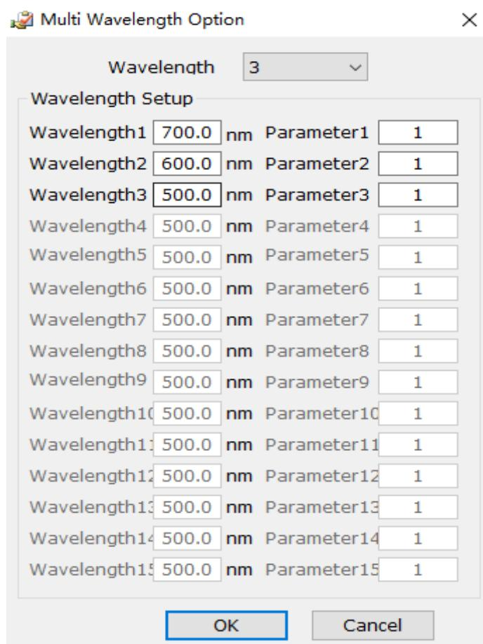
3. Enter wavelengths number, and enter measurement wavelengths and coefficient:
