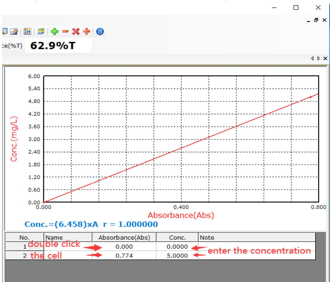
5. Put the sample into the light path, select the menu <operation> <Set Blank> or click the shortcut toolbar buttons [Set Blank], instrument will be set to the operating wavelength, and set blank 0.000 Abs/100.0 %T.
