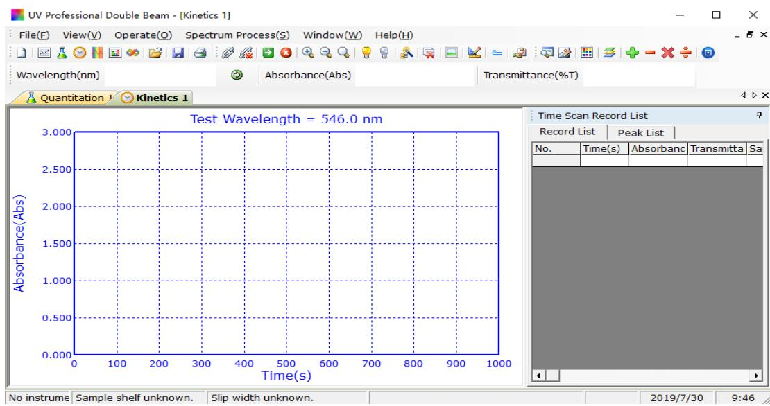
2. Click shortcut toolbar [ option], setup time scan parameters, select display mode, wavelength, start time, end time, time interval.
