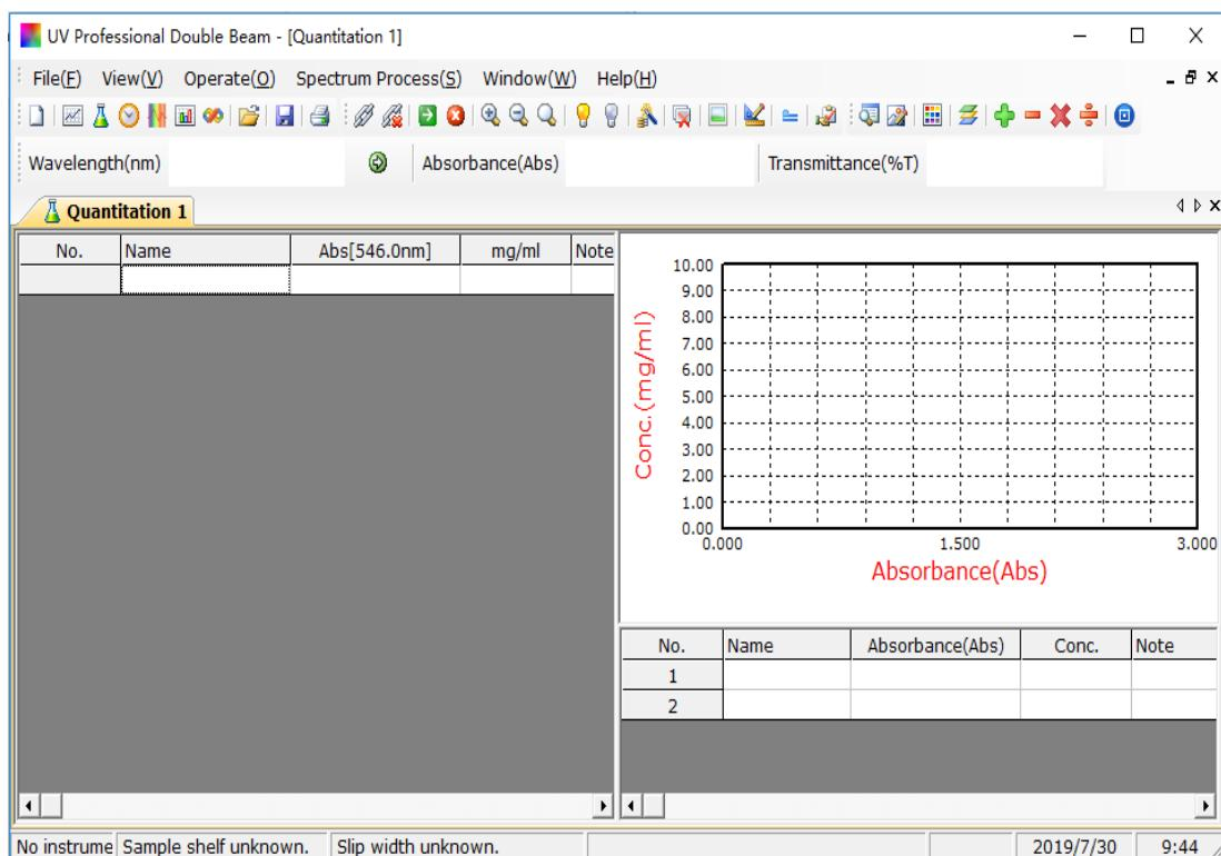
2. Shortcut toolbar [
