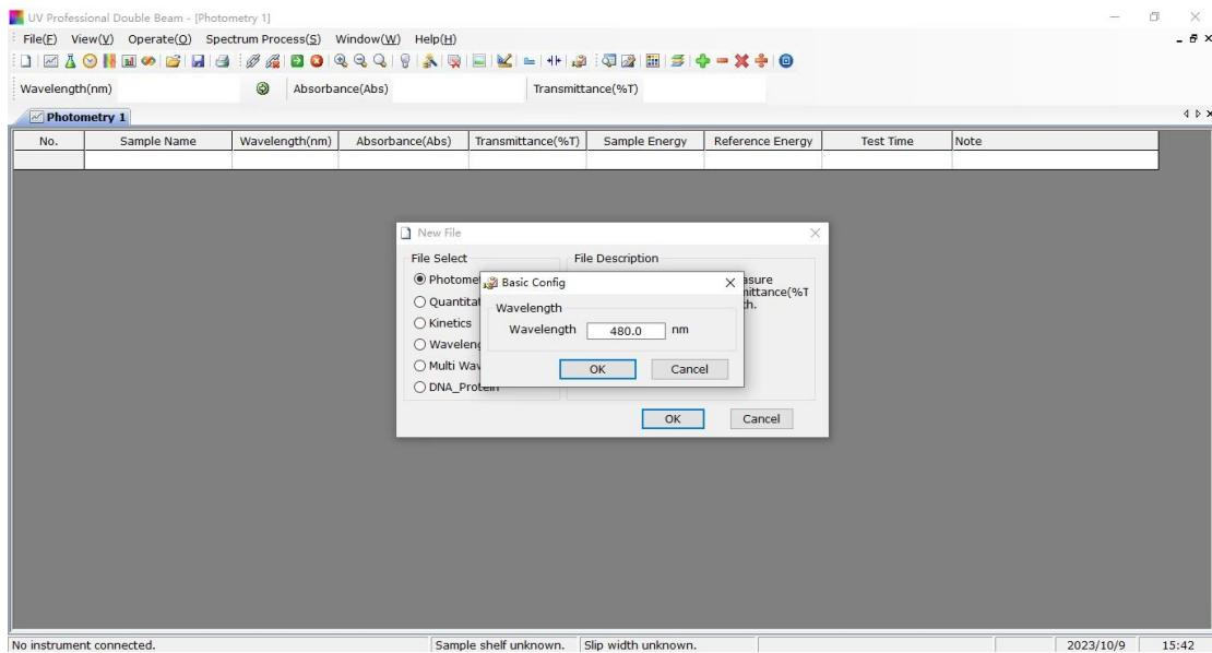
2. If you want to change the wavelength, press (option) to enter the test wavelength, press OK. Then the device will set it at the wavelength when doing blanking with blank solution.
