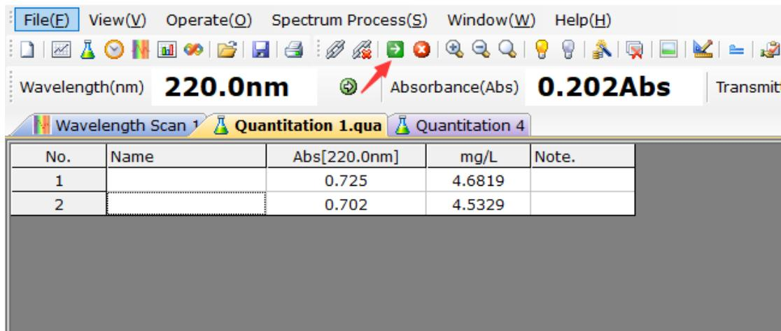
6. Put the samples into light path, select the main menu <operation> <start test> or click the shortcut toolbar buttons [ start test] to measurement the current absorbance data, calculate the concentration within the above formula, then display the data in the data list.
