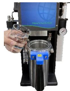
**7.8 Put the PTFE Insert into the Extraction Vessel and the Extraction Vessel into the instrument.**
