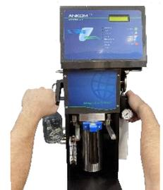
3.2 Use the Extraction Vessel Handle to pull the Extraction Vessel out.
