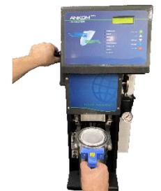
3.3 Remove the white PTFE Insert from the Extraction Vessel.
