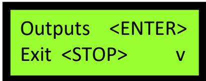
7. Press the STOP button on the Keypad to go back to the main Diagnostics screen (shown to the right).
