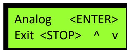
6. Press the STOP button on the Keypad to go back to the main Diagnostics screen (shown to the right).
