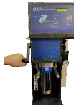
**IMPORTANT:** Before running the instrument, verify that the Extraction Vessel is locked in place by attempting to rotate the Main Handle upward. If it is not locked, repeat step 7.4 above.
