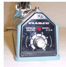
8. Seal the filter bag within 4mm of its open end. Keep the sealer arm down for 2 – 3 seconds after the red sealer light turns off (to cool the seal). The seal can be seen as a solid melted stripe along the top edge of the filter bag (as shown to the right). If the seal is not strong, re-seal the bag.
