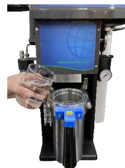
**7. Put the PTFE Insert into the Extraction Vessel and the Extraction Vessel into the instrument.**
