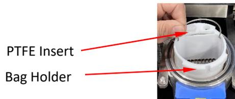
**7.7 Insert solvent into the Extraction Vessel.**
