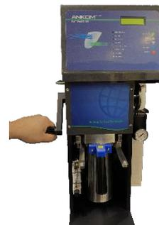
**IMPORTANT:** Before running the instrument, verify that the Extraction Vessel is locked in place by attempting to rotate the Main Handle upward. If it is not locked, repeat step 7.8.4 above.
