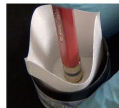
5. Pipette 1.5 – 2 g of liquid sample into the DE indentation in the filter bag. (Do NOT use more liquid sample than can be absorbed by the DE.)
