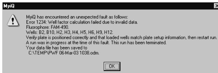
**Cause:** The plate from which you are attempting to collect well factors was not inserted into the reaction module, or is too dim to collect valid well factors.
