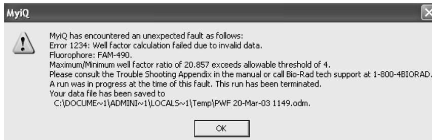
**Cause:** Invalid well factor data was collected. Either negative well factor values were recorded, or the highest to lowest well factor ratio exceeds 4.0. Thus, at least one well contains relatively low levels of fluorescence or deviates significantly from the rest of the wells on the plate you are attempting to collect well factors from.
