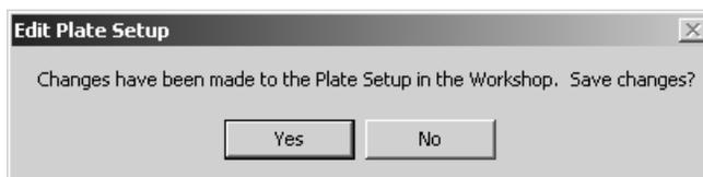
**Cause:** The currently opened plate setup has been edited in some way, but the changes were not saved before you chose to exit the software or to open another plate setup file.
