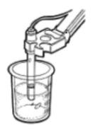
3. For long term storage, the probes can be stored dry or in distilled water.
