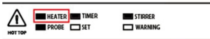
Note, however, that the HEATER LED will be turned on and off during the operation because the heater is automatically activated or deactivated to maintain the set temperature.
