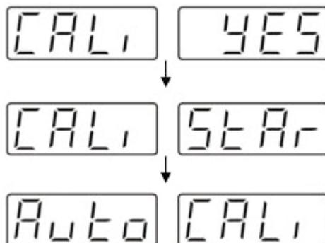
Step 4 : Terminate configuration mode as described in Configuration Mode. To cancel the auto-tuning during the process, turn off the main power switch. If cancelled, the Optimal Mode will be selected automatically with an alarm.
