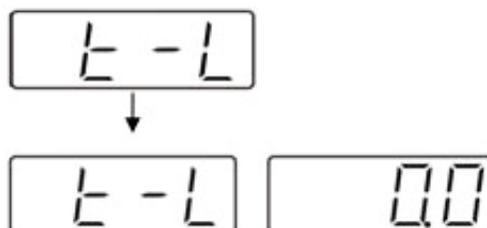
Step 3 : Change the limit to the desired value by turning the Stirrer Knob.
