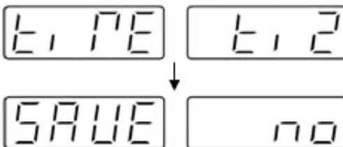
Step 4 : Save the desired timer mode by using the Stirrer Knob as shown below. [When you need to save the changes]
