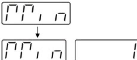
Step 3: Change the limit to the desired value by turning the Stirrer Knob and press the Stirrer knob.
