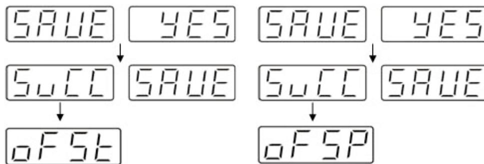
[OFST- Top plate offsetting]                      [OFSP- External temperature probe]
