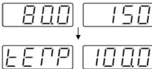
Step 2 : Select the desired temperature by turning and press the Heater Knob.
