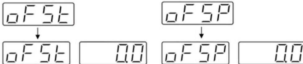
[OFST- Top plate offsetting]                      [OFSP- External temperature probe]
