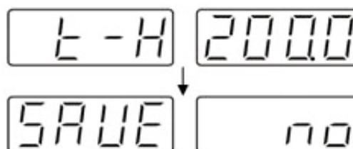
Step 4 : Save the desired limit by using the Stirrer Knob as shown below.
