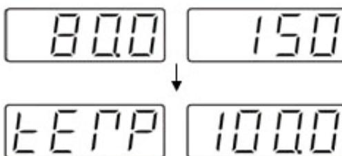
If you press the Heater Knob, set temperature is shown on the left. After 3 seconds, the mode will be escaped automatically.
