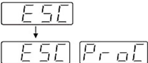
Note also that the configuration mode is automatically terminated if there is no button operation for more than 20 seconds.
