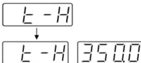
Step 3 : Change the limit to the desired value by turning the Stirrer Knob.
