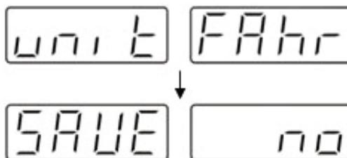
Step 4 : Save the selected temperature unit by using the Stirrer Knob as shown below.
