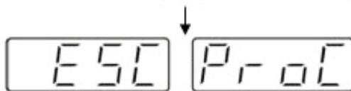
Or turn the stirrer knob clockwise until you get the following ESC display and then push it to confirm the termination as shown below:
