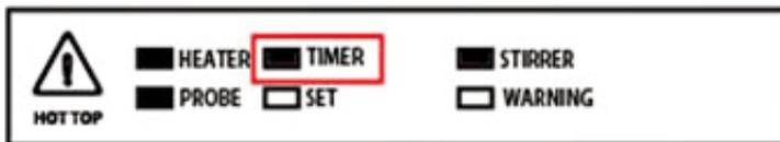
You can stop timer by pushing RUN/STOP Button during timer's activation. For both timer modes, the timer setting procedures are the same:
