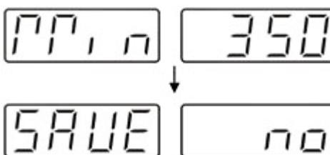
Step 4: Save it by using the Stirrer Knob as shown below.
