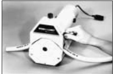
Figure #4. Adjust Occlusion
