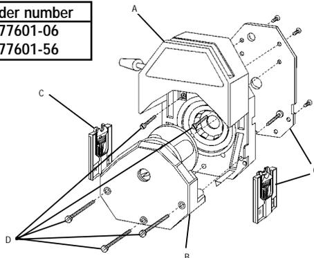
D. Mounting hardware for I/P EASY-LOAD pump heads.
