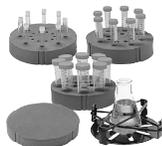
**3" Rubber Head Cover & 3" Head**- Designed for mixing irregular shaped objects.
