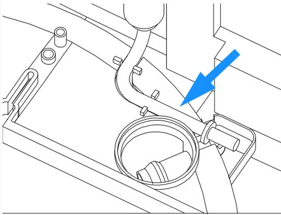
**14** Replace the heat exchanger assemblies, see "[Installing the Heat Exchanger Assemblies](#)" on page 84.
