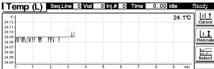
Press F6 key (**Select**). Here you can add additional online signals (maximum are 3). Additional signals could be also pressure or detector signals from other modules. Use the Right/Left arrows to switch between Available and Selected Signals. Use the F8 key (**Move**) to enter available signals into the box for selected signals or vice versa.
