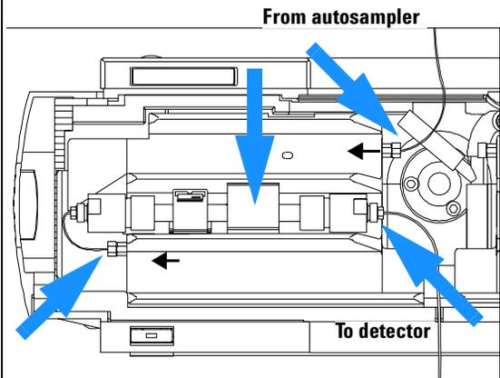
**4** Or place the column on the right heat exchanger assembly and connect the capillaries to the column.
