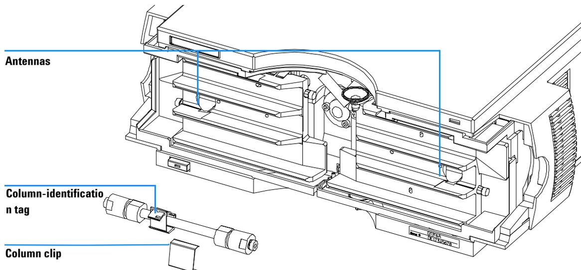
**Figure 28** Column-Identification System
