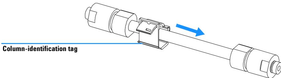
**Figure 29** Column-Identification Tag for Left Heat Exchanger
