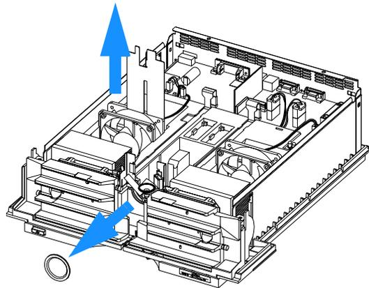
**2** Replace the valve into its location.
