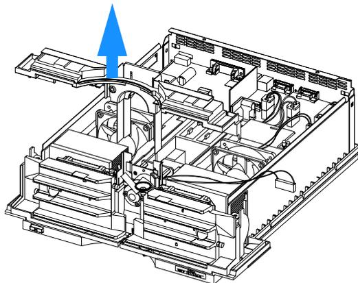
**8** Remove the Valve from its location.
