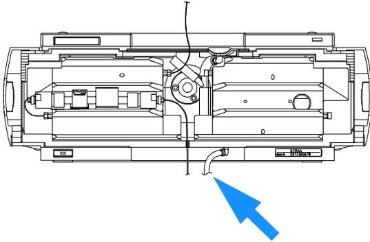
**7** Route tubings from modules above through the openings in the funnel holder (top) and the plastic bottom part. Remove small plastic plugs first.
