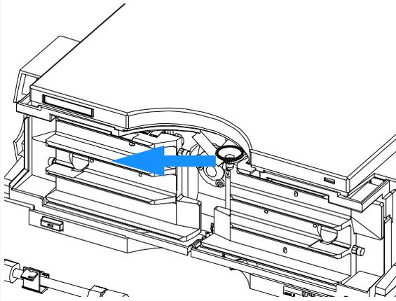
**3** Move the power lock across the power inlet and lift the clips on the rear of the cover.
