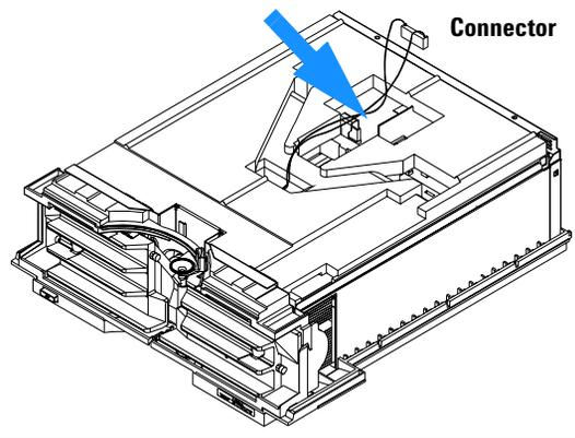
**3** Make sure that the foam is installed correctly and is located in the safety light switch.
