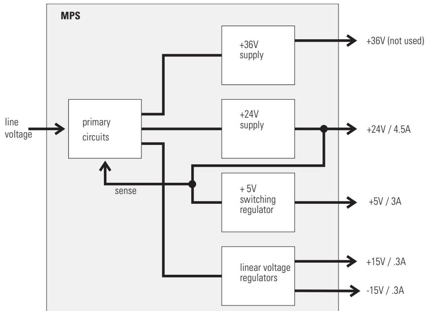
**Figure 42** Main Power Supply (MPS) Block Diagram
