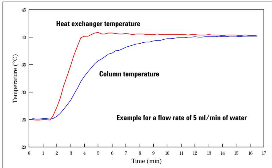
**Figure 27** Equilibration of Heat Exchanger and Column Temperature
