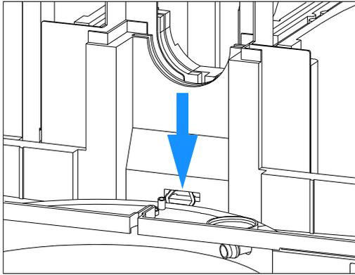
**12** Replace the clips (shown from the inside of the column compartment) on both sides using a flat screwdriver.
