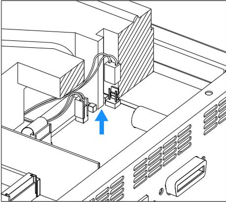
**8** Position of safety light switch on the main board when removing the foam.
