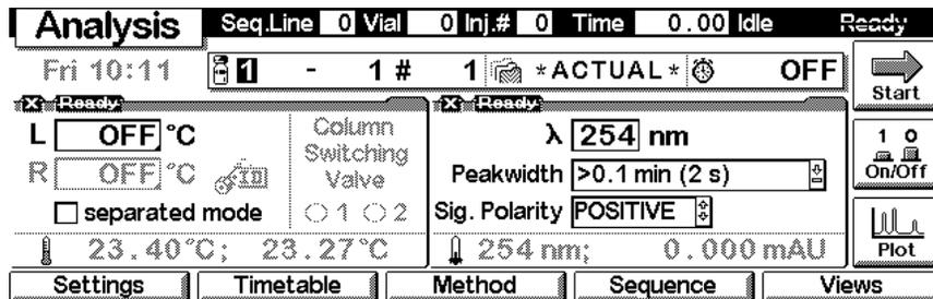
With the **Settings** key you open a pull-down menu where you can select the column compartment module.
