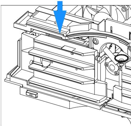
**6** Press down completely until it clicks into its holding position.
