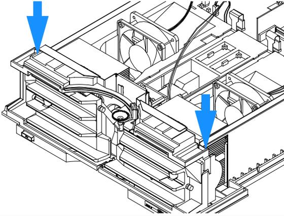
**3** Press against the rear of the Z-panel to release the metal plate from the guide and pull it carefully upwards.
