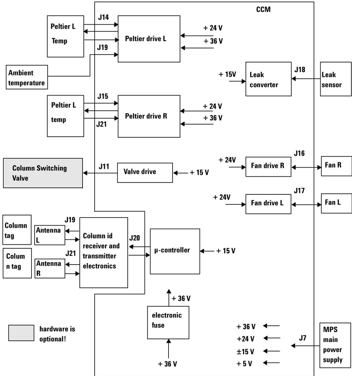
**Figure 38** Interconnection Diagram Column Compartment Main Board
