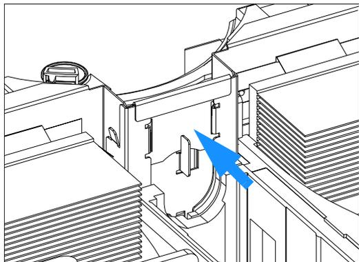
**5** Lift the Z-panel together with the top plastic panel half-way out of the guide.
