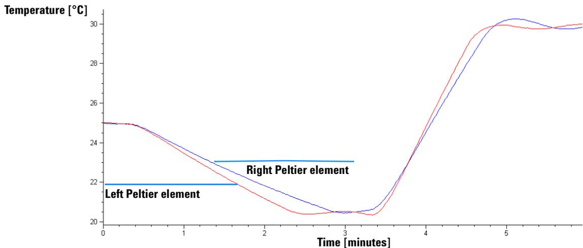
**Figure 7** Typical Thermostat Function Test Profile
