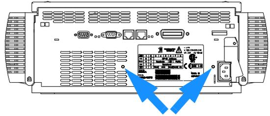
**17** Press down the power switch light pipe to remove it from the coupler.
