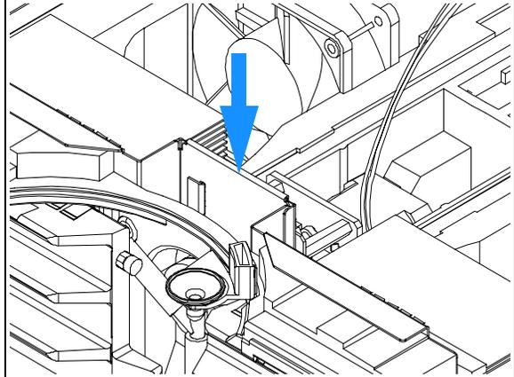
7 Fix the Z-panel with the two screws.
