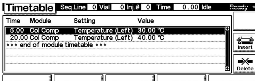
Press the F7 key (**Insert**) to add a timetable events. Use the F6 key (**Done**) to view the entered lines of the timetable.
