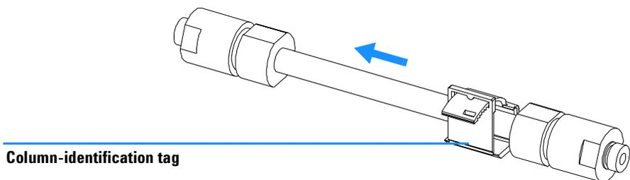
**Figure 30** Column-Identification Tag for Right Heat Exchanger
