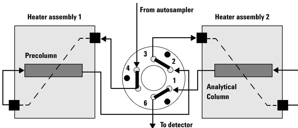
**Figure 35** Precolumn Back-flushing
