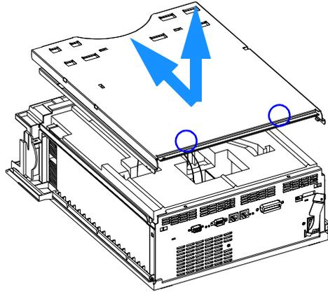
6 If installed, disconnect the connector of the column switching valve from column compartment and remove the top foam.
