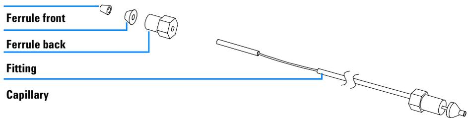
**Figure 1** Capillary (Column-Heat Exchanger) Parts
