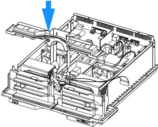
**4** Carefully plug the temperature sensor into the rear of the top plastic panel.
