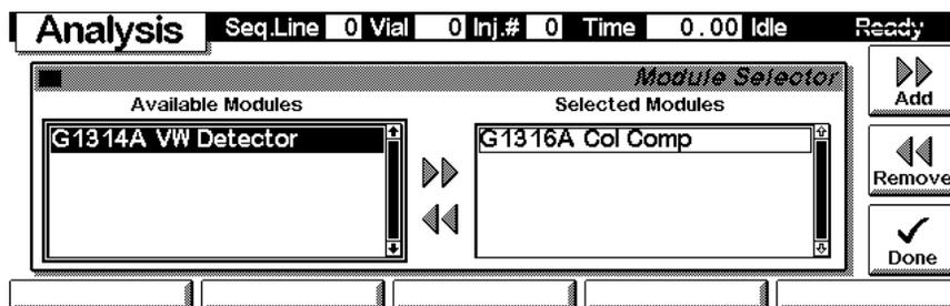
Here, e.g. the variable wavelength detector parameters are shown on the display as well. The number of parameters on the display are restricted as additional modules are added. Maximum 4 modules are shown automatically. If more modules are in the system, you have to choose in Setup view.
