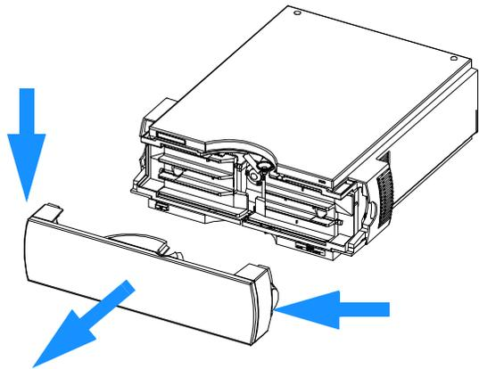
**2** Pull the leak funnel out of the leak funnel holder.
