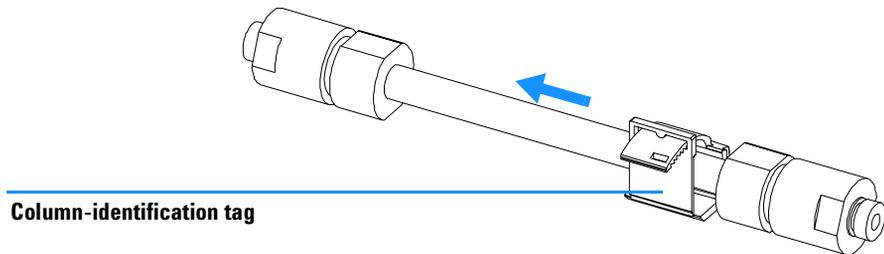
**Figure 13** Column-Identification Tag for Right Heat Exchanger
