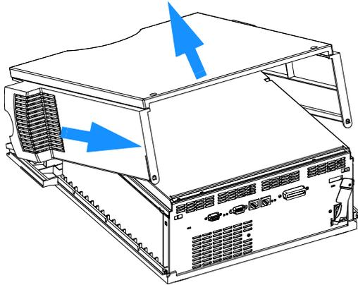
5 Unscrew the screws at the rear of the top plate, slide the plate towards the front and remove it.
