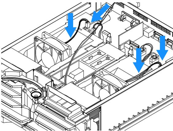
**5** Replace the foam section, the top cover and front cover, see "[Installing the Foam and the Top Cover](#)" on page 96.
