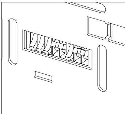
**Figure 41** 8-bit Configuration Switch
