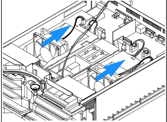
**4** Reconnect the fan assembly to the processor board and check that the cable of the left fan is correctly in the foam channel to assure correct closing of the foam parts.
