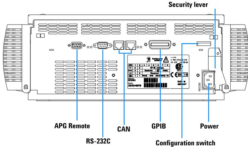
**Figure 5** Rear View of the Thermostatted Column Compartment
