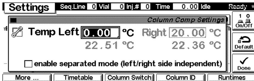
Use the **m**-key for the context sensitive menu. The **Status** command pulls up a monitor screen displaying signals and spectra as programmed. **Reset** will load the TCC default parameters.
