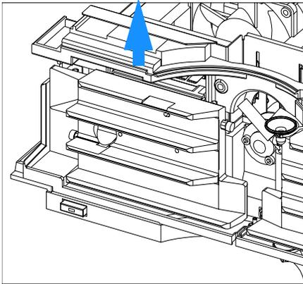
**5** Locate the ambient temperature sensor in the top plastic part and push it towards the rear.
