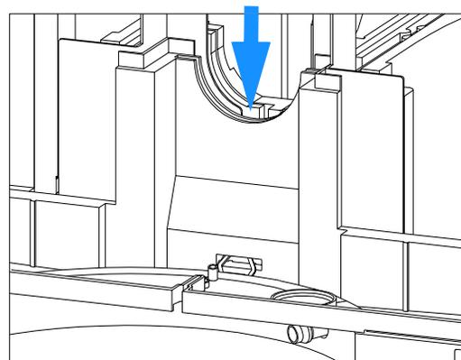
**10** Replace the leak base into the cabinet until it clicks into the cabinet. Insert the right side first.
