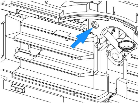
**7** Carefully remove the ambient temperature sensor plugged into the rear of the top plastic panel.
