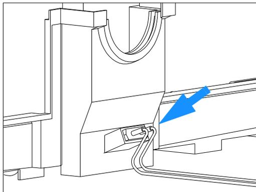
**9** Route the leak sensor cable through the z-panel into the left foam channel.
