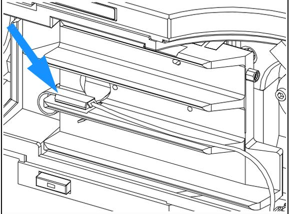
**5** Route the sensor wire through the slit in the leak tray.
