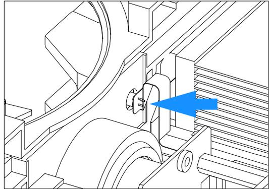
**Ensure that the ambient temperature sensor is completely plugged into the rear of the top plastic panel.**
