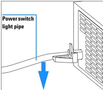
**18** Remove the power supply completely.
