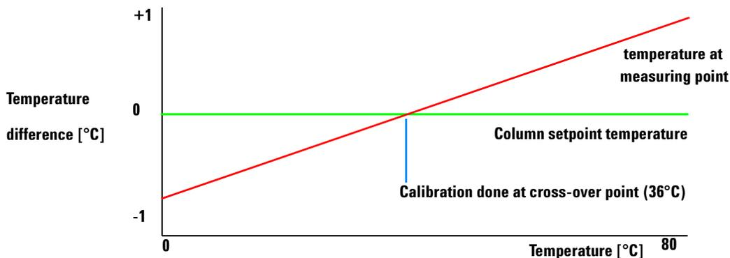
**Figure 8** 1-Point Calibration at the Temperature Cross-Over Point.
