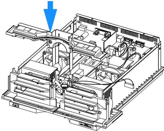
**4** Carefully plug the ambient temperature sensor into the rear of the top plastic panel.
