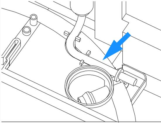
**2** Replace the heat exchanger assembly. A screwdriver might be helpful to insert the silicon isolation.
