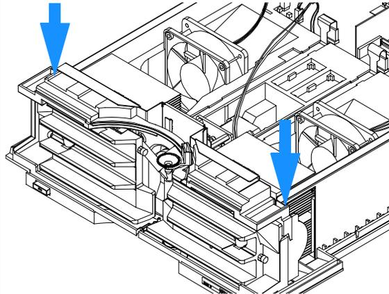
**4** Press against the rear of the Z-panel to release the metal plate from the guide and pull it carefully upwards.
