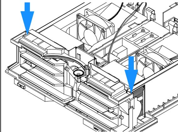
8 Reconnect the heat exchanger cables to the processor board and the grounding connection of the column switching valve.
