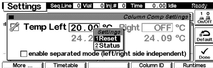
Use F1-key (**More**). You can enter special TCC setpoints that enables the analysis either with any temperature or within a specified range.
