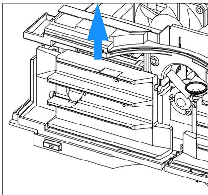
**6** Locate the ambient temperature sensor in the top plastic part.
