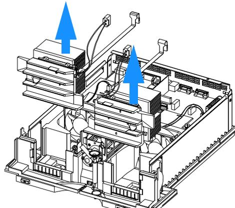
**The repair level of the heat exchanger assemblies is the complete assembly.**
