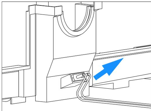
**8** Replace the leak sensor assembly into the leak base.
