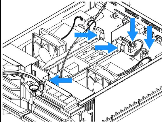
9 Carefully replace the heat exchanger cables into the foam channels.
