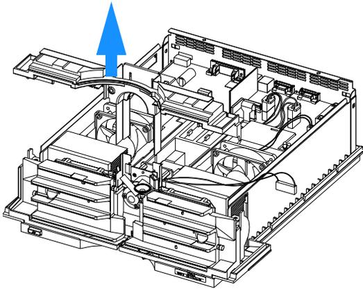
**9** Remove the heat exchanger assembly.
