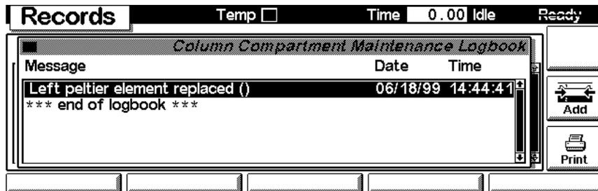
Use the F7 key (**Add**) to add new maintenance activities. If an activity is not listed, you can type the activity into the line “Add” using the control modules key pad.
