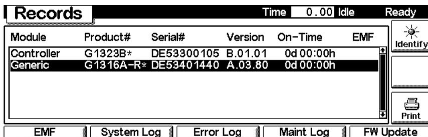
Use the F5 key (**FW Update**) to enter the Update section. Select the a file from the PCMCIA card (1316nnnn.DLB) and press execute. When the update has finished, press F7 key (**Transfer**) to return the module into the normal mode (LED on module should stay yellow).
