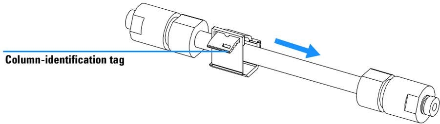
**Figure 12** Column-Identification Tag for Left Heat Exchanger
