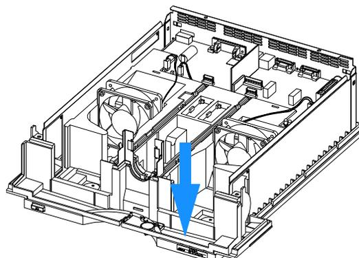
**11** Position the leak sensor so that it does not touch the bottom of the leak base.
