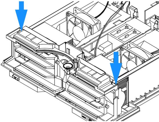
8 Reconnect the grounding connection of the valve at the Z-panel.
