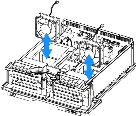
**3** The arrow on the fan should correspond with the direction of air flow which is from the front to the rear of the column compartment.
