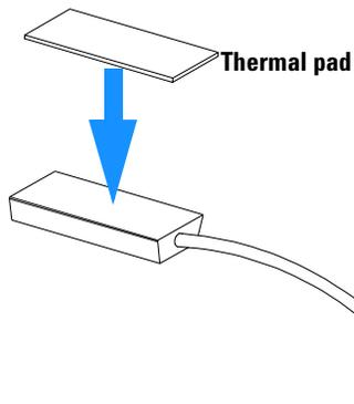
**2** Insert the temperature sensor into the spring. Ensure the face of the thermal pad faces downwards.
