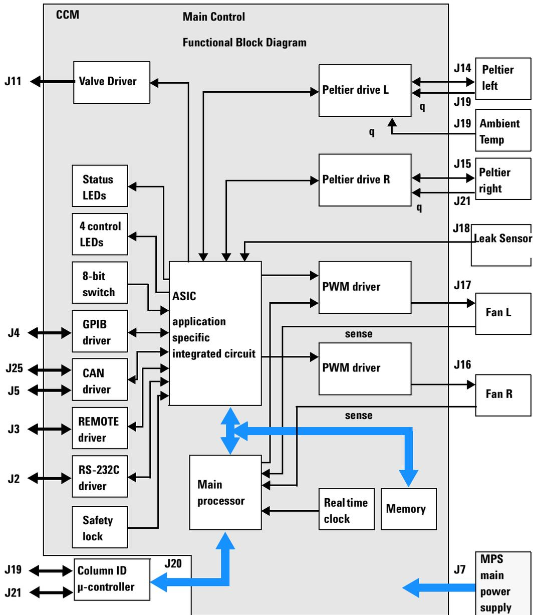
Figure 37 Block Diagram Column Compartment Main Controller Functionality
