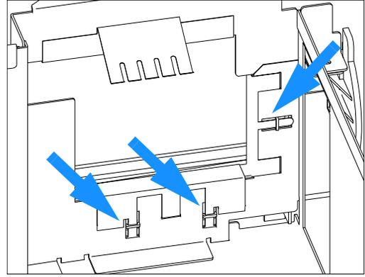
**13** Replace the leak tubing assembly into its location on leak base. Ensure that it keeps in this position during the next steps.
