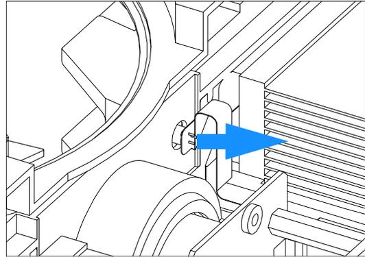
**8** Carefully pull out the top plastic panel together with the Z-panel completely.
