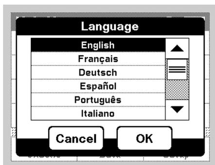
1. With the instrument off, press the **Power** key and hold it down until the language selection screen appears.
