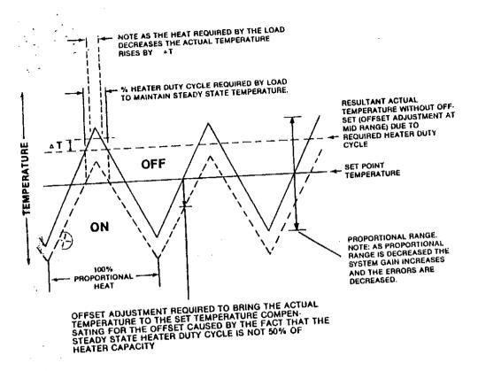
The graph summarizes the relationship between proportional and offset control. The shaded areas show how heat delivered to load is changed (proportionally) in response to temperature measurements.
