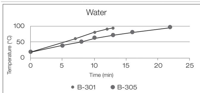
$\Delta T_{70\text{ }^{\circ}\text{C (water)}}$  : B-301 -> 13 min; B-305 -> 22 min
