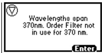
Figure 3-19 Dual Wavelength 370 nm Threshold Warning Message
