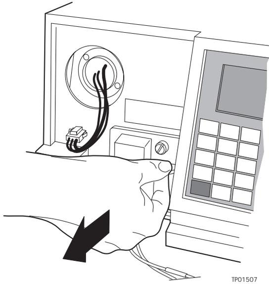
Figure 4-3 Removing the Flow Cell Assembly
