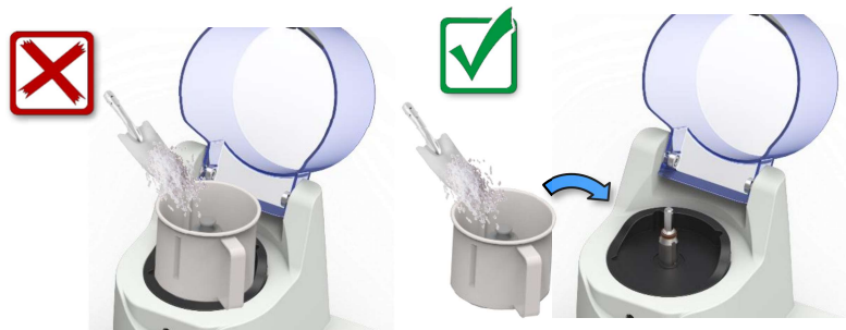
Fig. 4: Correct filling when grinding using dry ice and sample
