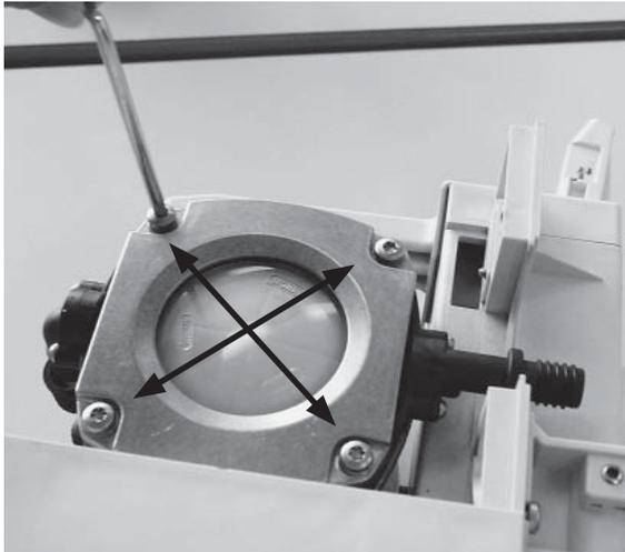
Fig. 7.2: Disassembling and reassembling the valve heads
