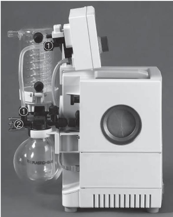
Fig. 5.6: Vacuum connection to the Easy- and LabVac
