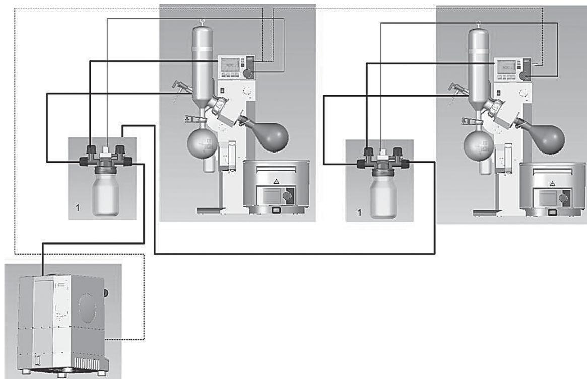
Fig. 5.8: Complete system connection with two Rotavapors
