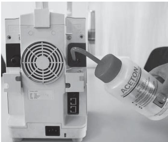
Fig. 7.1: Cleaning the valve head with acetone
