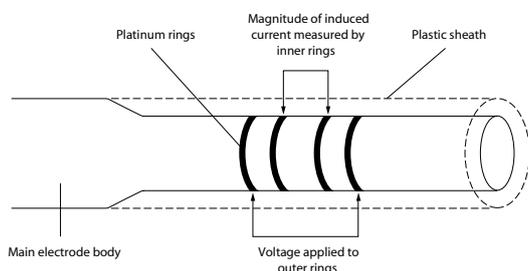
The STCON3 utilizes the 4-ring potentiometric method for measuring conductivity, which incorporates a series of four stainless steel rings formed into the probe shaft. This design completely eliminates polarization, which occurs with the 2-plates amperometric method. Furthermore, without polarization the probe can measure a wider range of conductivity values because it does not suffer from electrolysis.
