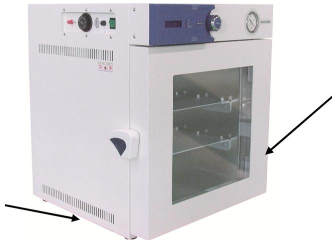
5. The product should be positioned in a location where it has enough space for ventilation and prevention from fire. The recommended distance of each side is minimum 20cm from the back wall, 100cm from the side walls and ceiling respectively.
