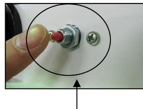
2) Remove the red cap of the Protector by turning it to the left and press the switch once. Then, you should hear the 'click' sound, the protection will be released and the unit will work.
