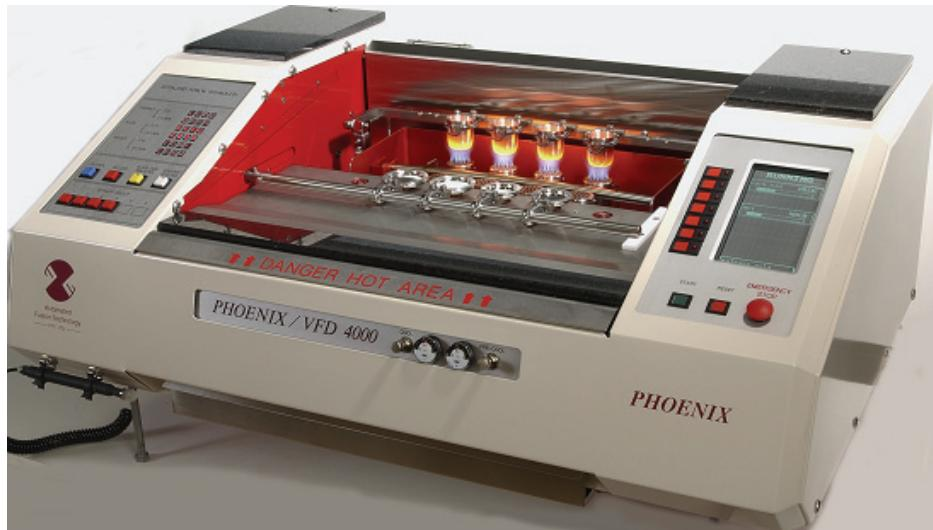
The Phoenix series of Fusion Machines are designed to allow the preparation of permanent and homogeneous fused beads under accurately reproducible conditions.
