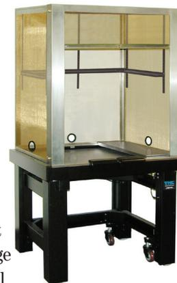
frame and bronze-mesh material and mounts to a required full-perimeter enclosure. Our 40 in. tall Faraday Cage includes a 2 in. diameter hole in the base of the side and rear panels. This feature eases cable interface to the interior of the cage. A new version of our armrest pads that is compatible with our cages. They are identical to our non-Faraday Cage pads but adhere with Velcro.
