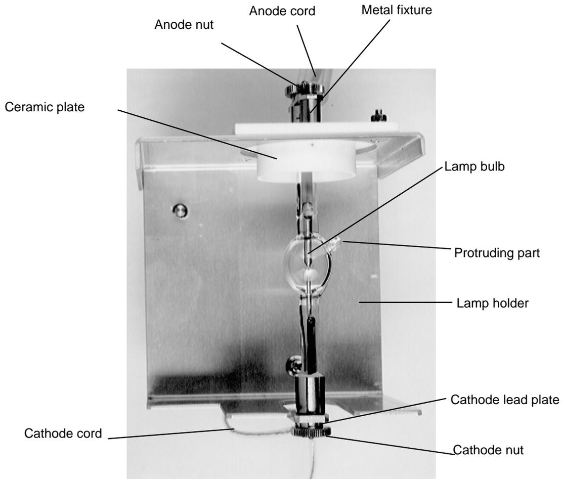
Figure 15 Xenon Lamp Mounted in Holder
