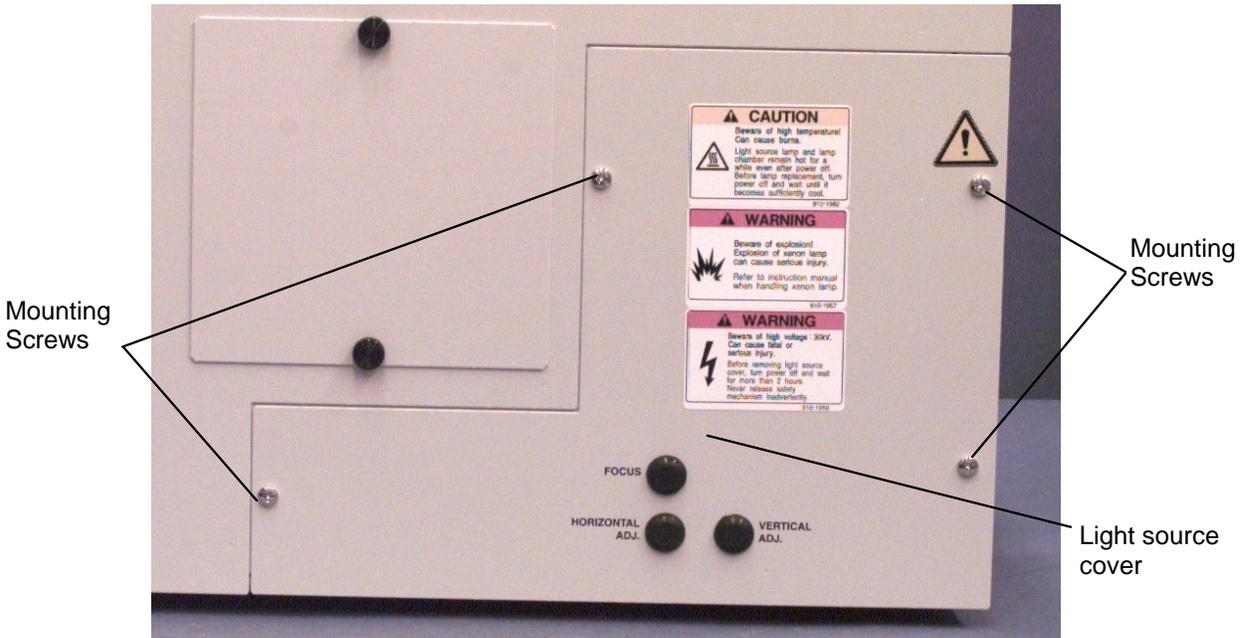
Figure 12 Removal of Light Source Cover
