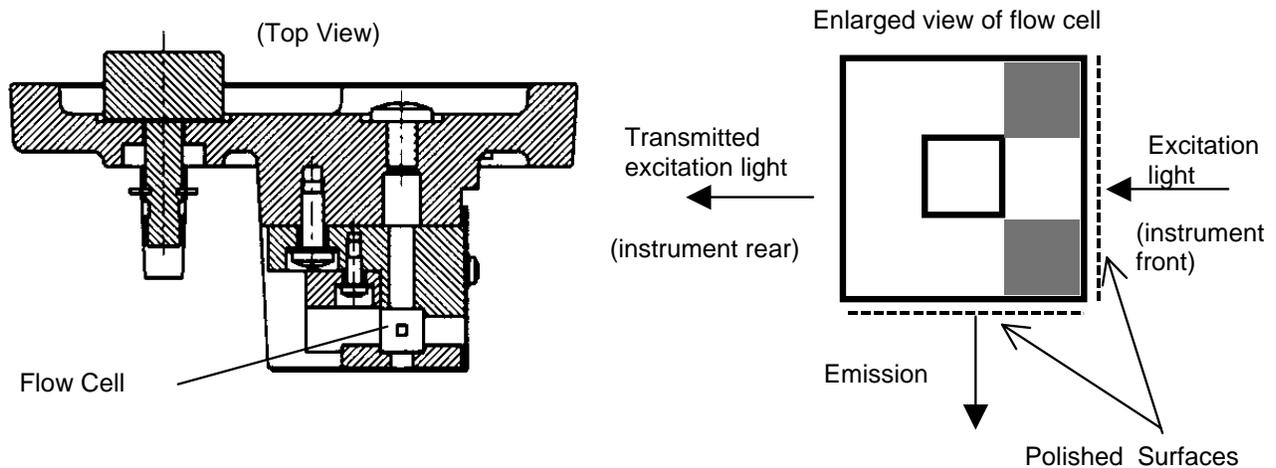
Figure 23 Assembly of Flow Cell Unit
