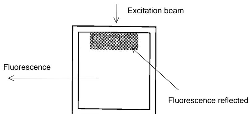
*Figure 26 Sample Containing Extremely High Concentration*
