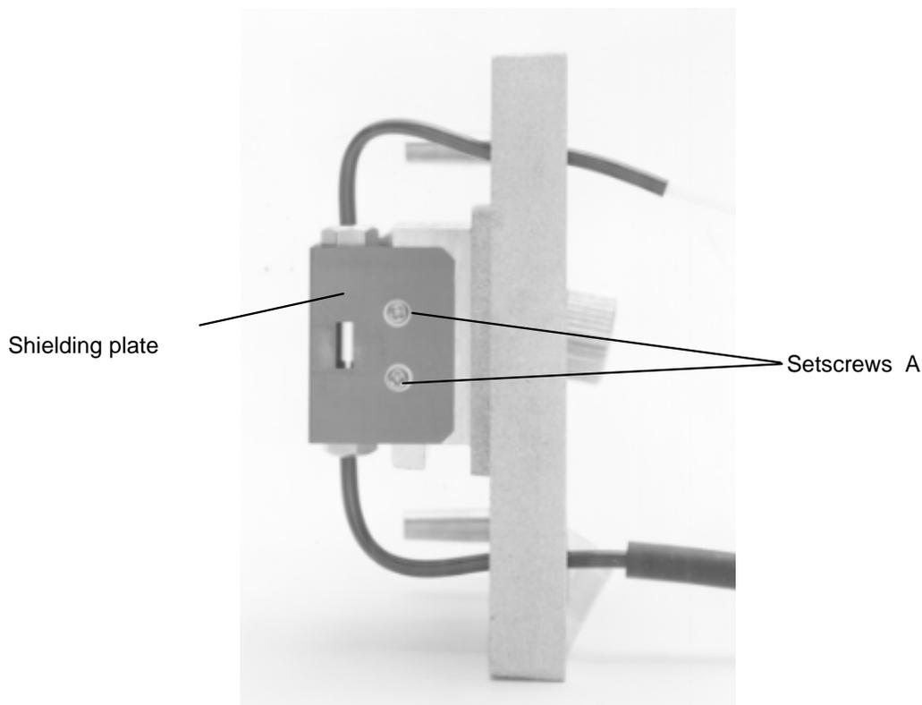
*Figure 21 Flow Cell Unit*
