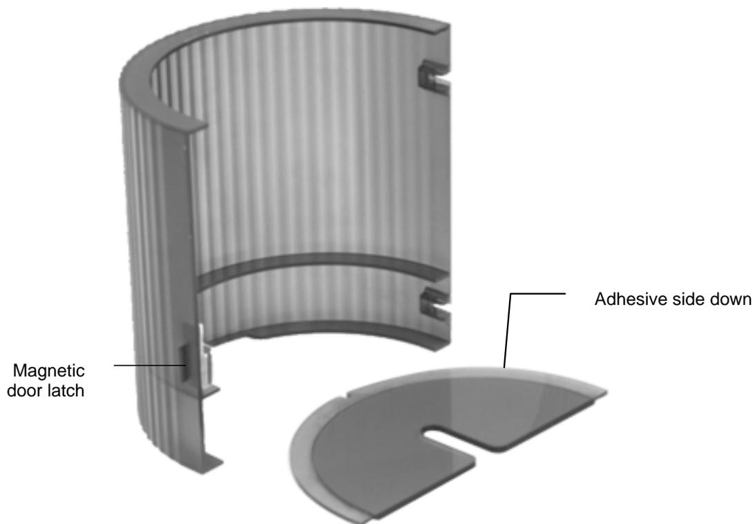
*Figure 3 Door and Door Cap Orientation*
