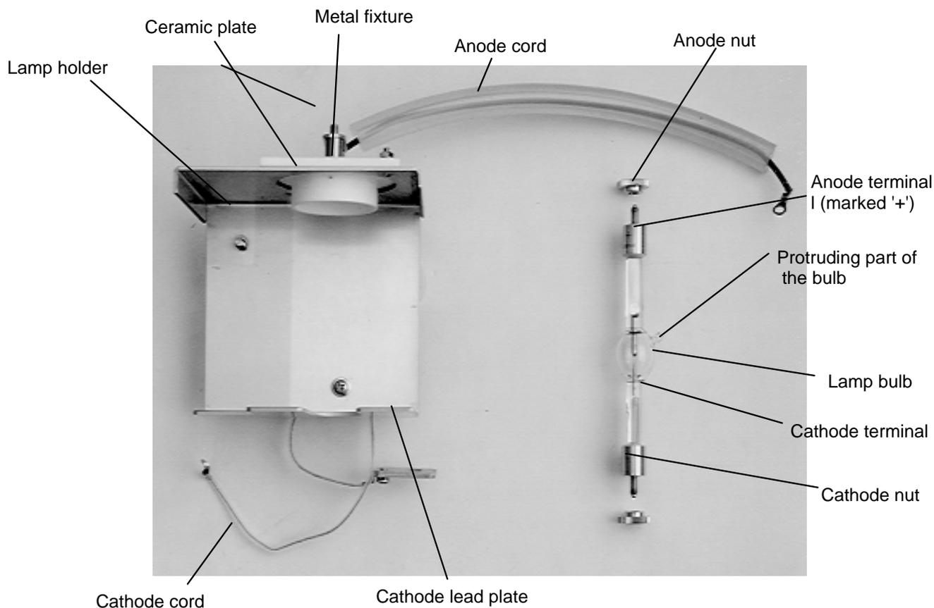
*Figure 13 Xenon Lamp and Its Holder*
