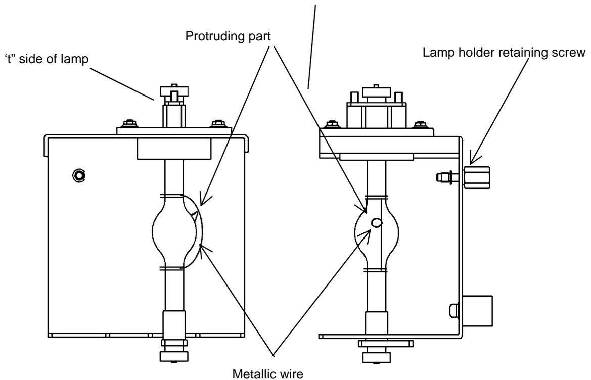
*Figure 14 Protrusion of Lamp Bulb*
