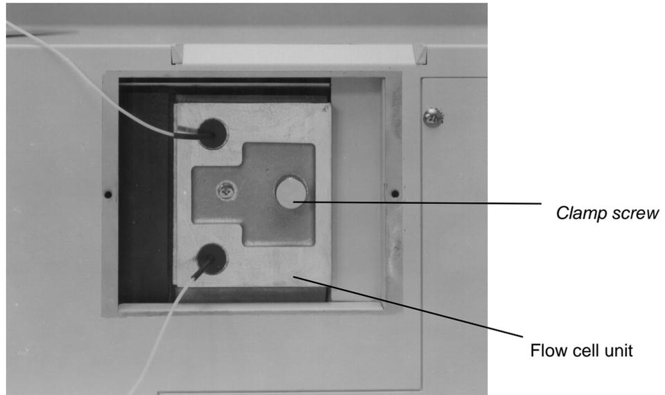
Figure 20 Flow Cell Cleaning
