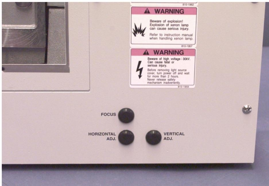
*Figure 18 Adjusting the Lamp Position*
