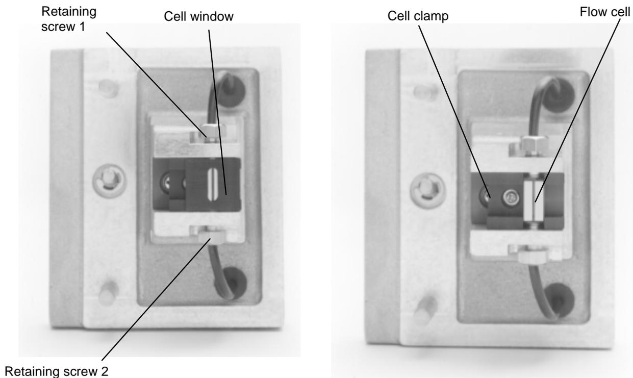
*Figure 22 Disassembly of Flow Cell Unit*
