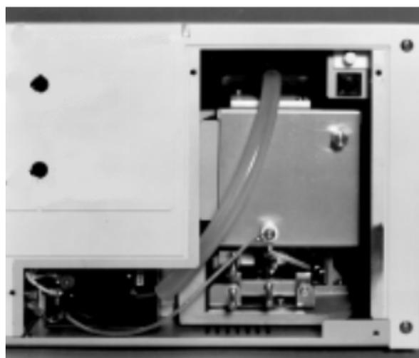
*Figure 17 Connecting the Anode and Cathode Cables*
