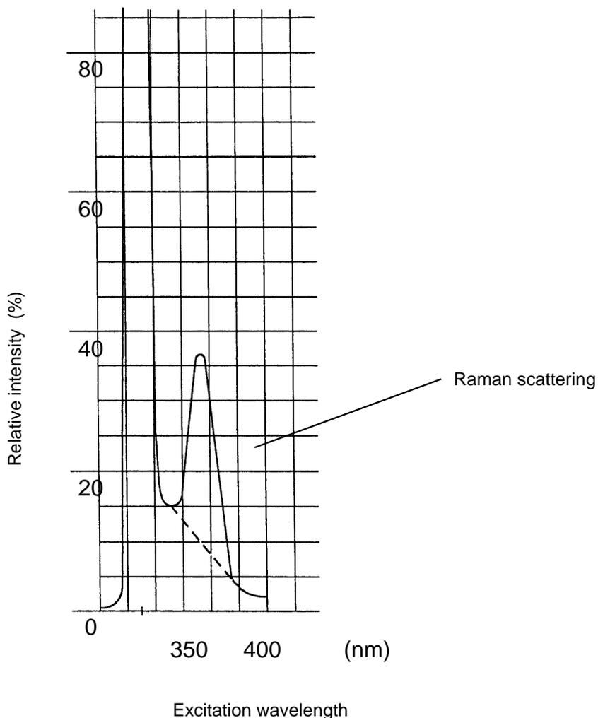
Figure 25 Raman Spectrum of Water
