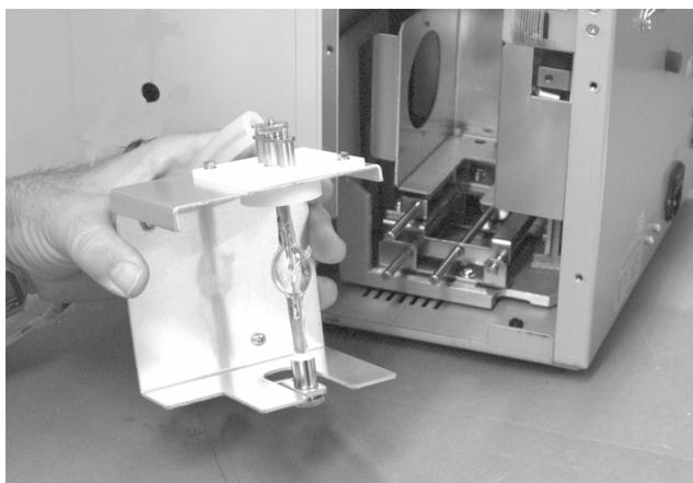
*Figure 16 Mounting the Lamp Holder*
