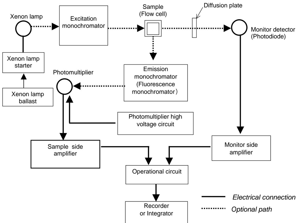
Figure 7 Functional Block Diagram
