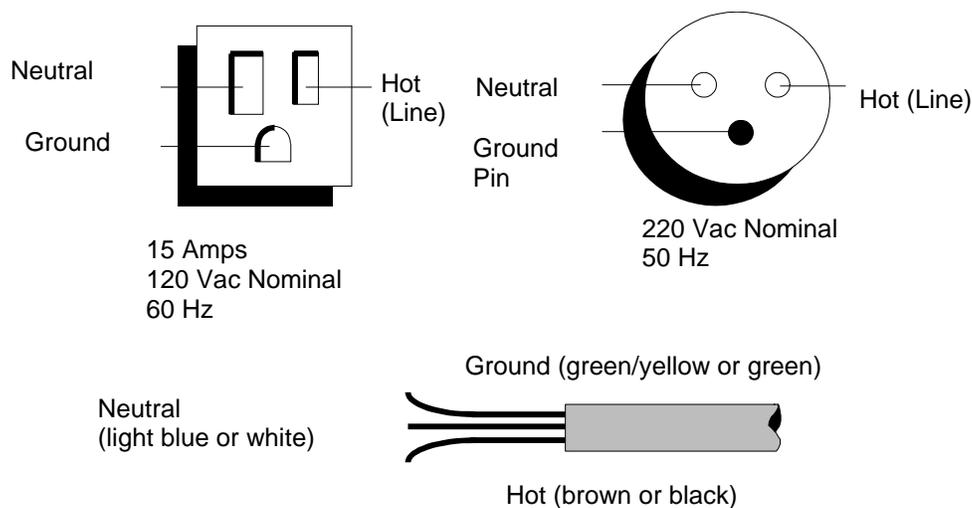
Figure 2 Power Receptacle Polarity
