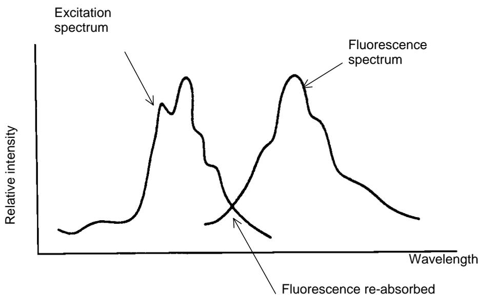
Figure 27 Re-absorption of Fluorescence
