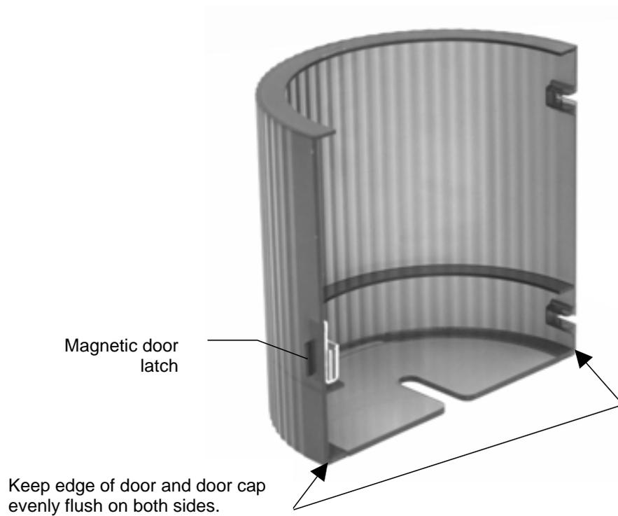
*Figure 4 Door and Door Cap Assembly*
