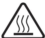
Caution : hot surface ! In normal operation, the pump surface temperature can exceed 80°C. There is a risk of burning. Switch off the pump and let it cool down before any intervention or take appropriate precautions.
