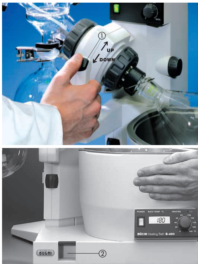
Picture 24: Lowering and raising the evaporating flask
