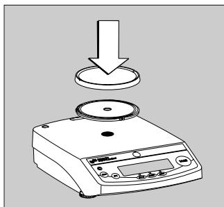
Instruments with a round weighing pan
