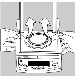
On analytical balances remove and clean the weighing pan as follows:
