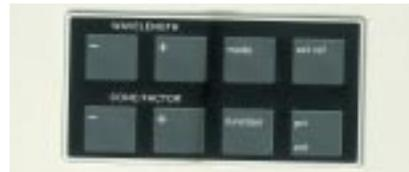
**Wavelength:** The -Wavelength+ keys are used to select operating wavelength. Pressing both keys at the same time performs a quick peak check scan 10 nm about the current wavelength.
