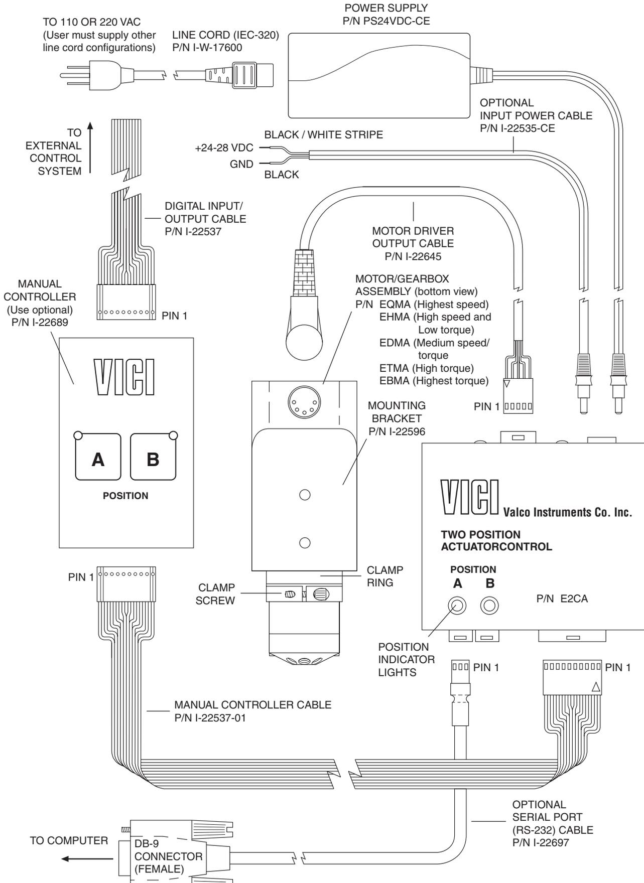
**Figure 1: Actuator and controller connections**
