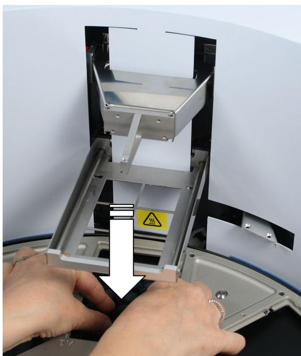
**Figure 4–47.** Pressing the heating block into place
