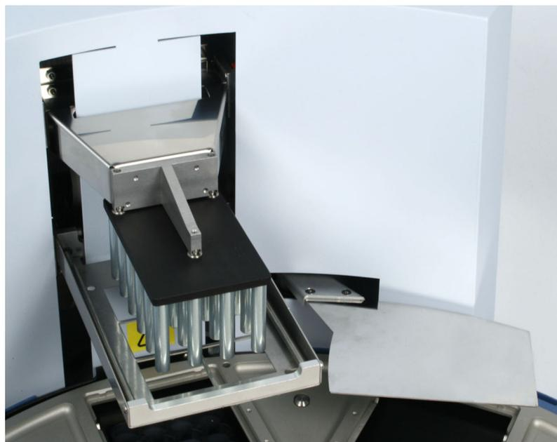
**Figure 3–24.** KingFisher Flex head for KingFisher 24 deep well plate fitted
