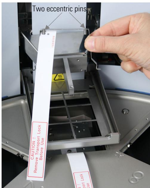
**Figure 3–11.** Tip comb holder transport lock removed
