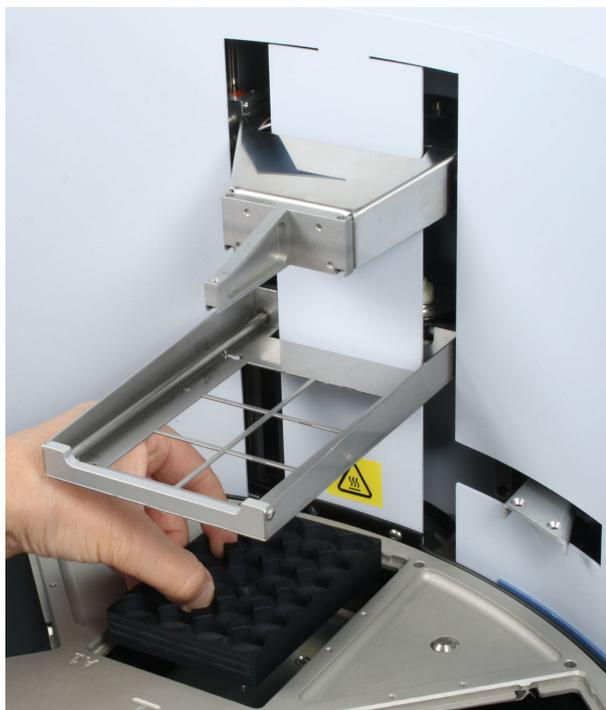
**Figure 4–46.** Inserting the heating block
