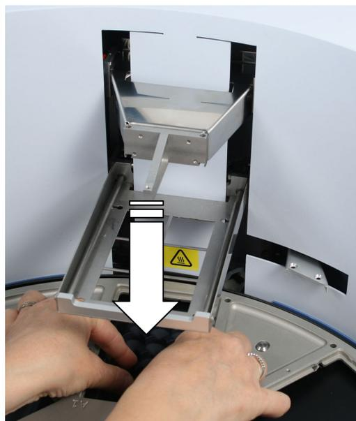
**Figure 3–16.** Pressing the heating block into place
