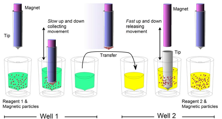
**Figure 2–7.** Inverse magnetic particle processing
