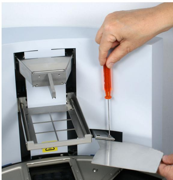
**Figure 3–20.** Fastening / loosening the shield plate
