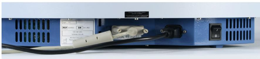
**Figure 3–14.** Mains supply cable and serial cable connected
