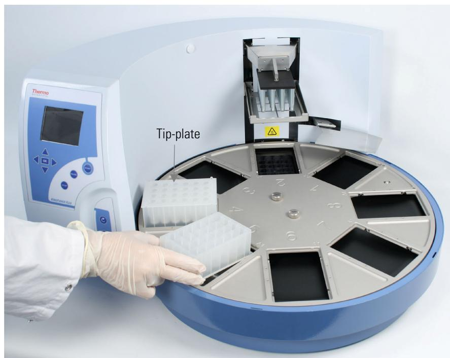
**Figure 4-41.** Loading the plates
