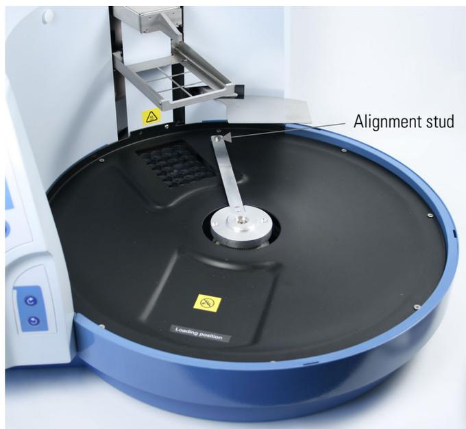
**Figure 5–51.** Black spill shield exposed for cleaning
