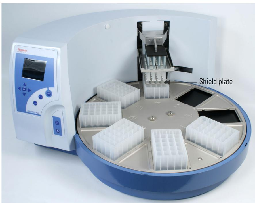
**Figure 4-44.** Shield plate in function
