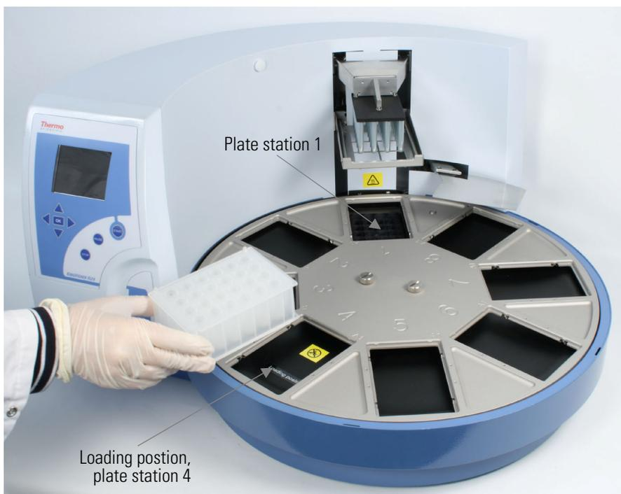
**Figure 4–39.** Combining the tip comb and KingFisher plate (B)
