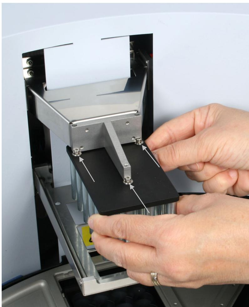
**Figure 3–23.** Inserting the KingFisher Flex head
