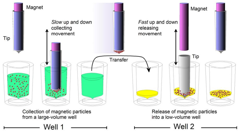
**Figure 2–8.** A concentration step during magnetic particle processing
