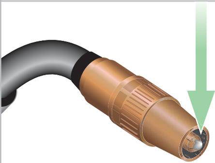
*ProStar* conduits reduce pull tension issues that are associated with weld wire burn-backs at the contact tip.
