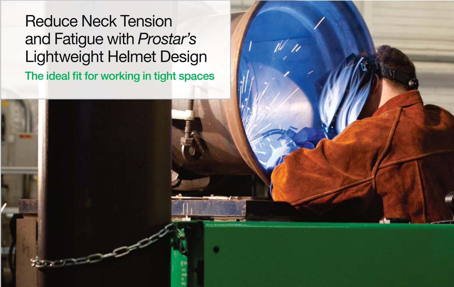
Both *ProStar* welding helmets feature an extended front that increases throat protection against sparks, slag, & fumes
