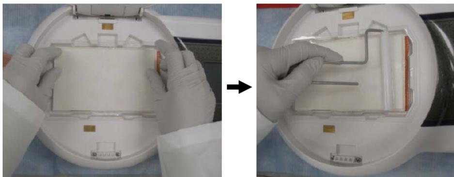
14. Remove and discard the white plastic separator from the Top stack.
