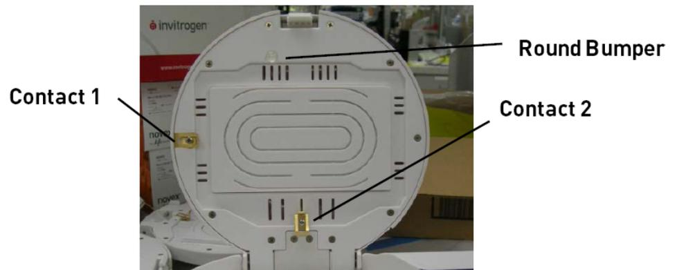
2. Hold the Lid with one hand, and remove the screw holding Contact 1. Discard both the screw and the contact.
