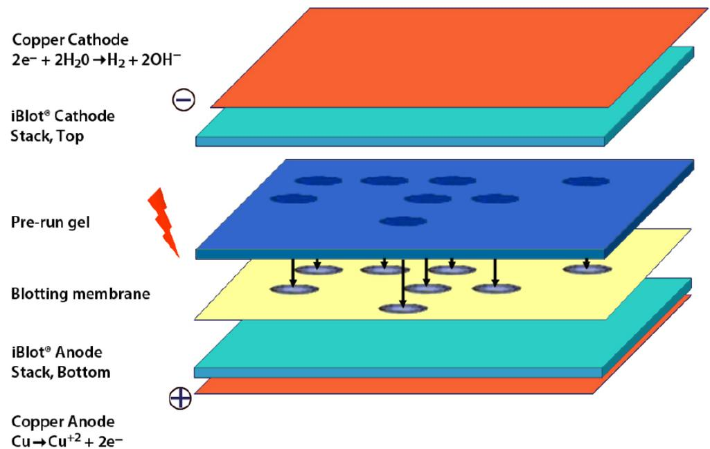
After the stack is assembled on the iBlot™ 2 Gel Transfer Device, and the appropriate Method is selected, the run is initiated. Complete transfer of proteins from the gel to the blotting membrane is accomplished in approximately 7–8 minutes. The rapid transfer without the need for external power supply or pre-made buffers is possible due to the following features of the iBlot™ 2 Dry Blotting System:
