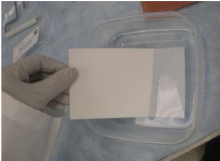
13. Place the presoaked iBlot™ Filter Paper on the pre-run gel. Use the Blotting Roller to remove any air bubbles between the filter paper and gel.
