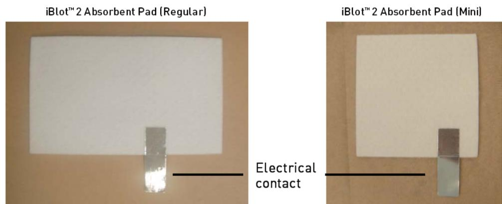
When properly assembled, the electrical contact of the iBlot™ 2 Absorbent Pad is aligned with the corresponding electrical contacts on the blotting surface of the iBlot™ 2 Gel Transfer Device to allow completion of the electrical circuit. See “iBlot™ 2 Transfer Stack specifications” on page 55 for dimensions of the iBlot™ 2 Absorbent Pad.
