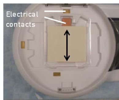
5. Ensure there are no bubbles between the membrane and the transfer stack. Remove any trapped air bubbles using the Blotting Roller.
