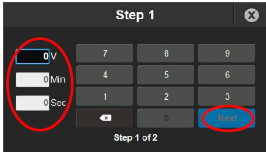
5. Select **Done** after programming the final step, and the entire Method is displayed. Select **Next** and proceed to to “Save a Custom Method” (“Save a custom method” on page 38).
