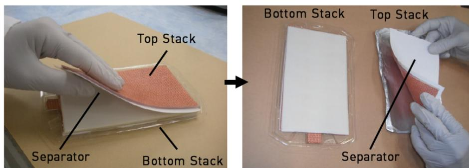
4. Place the Bottom Stack **with the plastic tray** directly on the blotting surface. Align the tray in the center of the blotting surface according to the type of iBlot™ 2 Transfer Stack being used.
