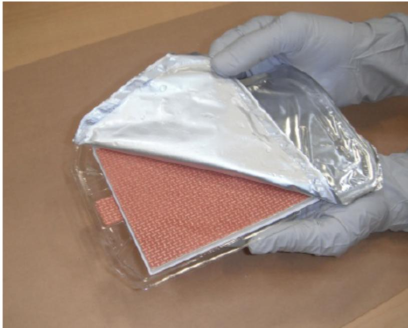
3. Separate the Top Stack and set it to one side of the bench with the transfer gel layer facing up. **Keep the Bottom Stack in the transparent plastic tray.**
