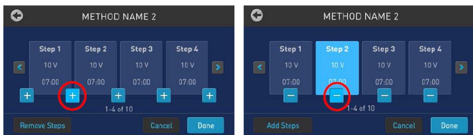
4. If a step is added, a screen appears to enter the desired voltage and time for that step. After the values are added, select **Done** to return to the Edit Method screen.
