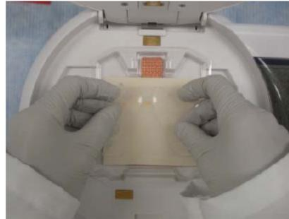
11. Use the Blotting Roller to remove any air bubbles between the gel and the membrane.
