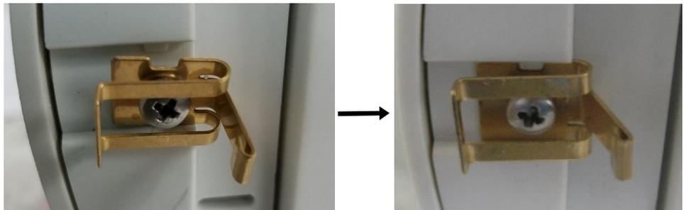
8. Place a screw through the hole in one of the contacts. Position the contact/screw onto the Contact 2 location. Turn the screw with a screwdriver until it is hand-tight.
