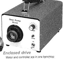
case. Adjust speed with front-panel potentiometer or by remote control. A 1/4" phone jack port accepts a 4 to 20 mA input signal. Remote control linearity is better than ±3% FS. Dimensions: 5.4"H x 6.4"W x 11.4"L. Shpg wt: 10 lbs (4.5 kg).
